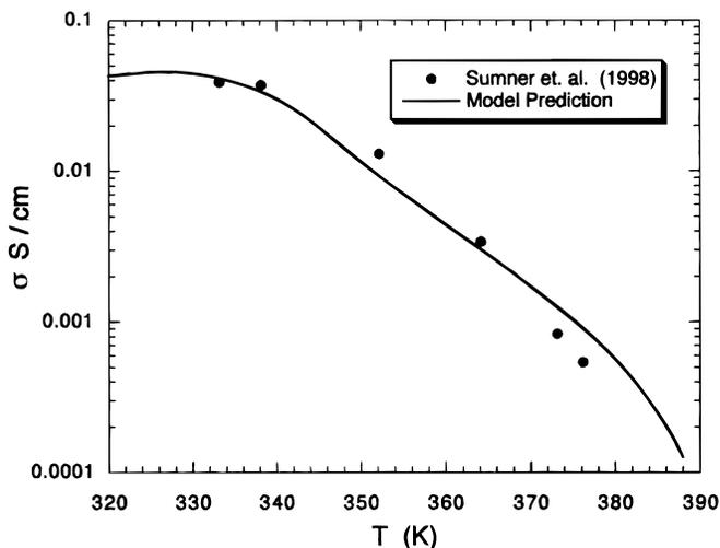
**Figure 6.** Effect of temperature on conductivity of Nafion 117 at a fixed partial pressure of water ( $2.0 \times 10^4$  Pa, *i.e.*, humidifier temperature =  $333$  K). The data of Sumner *et al.*<sup>34</sup> are plotted along with model predictions for parameters listed in Table I.
