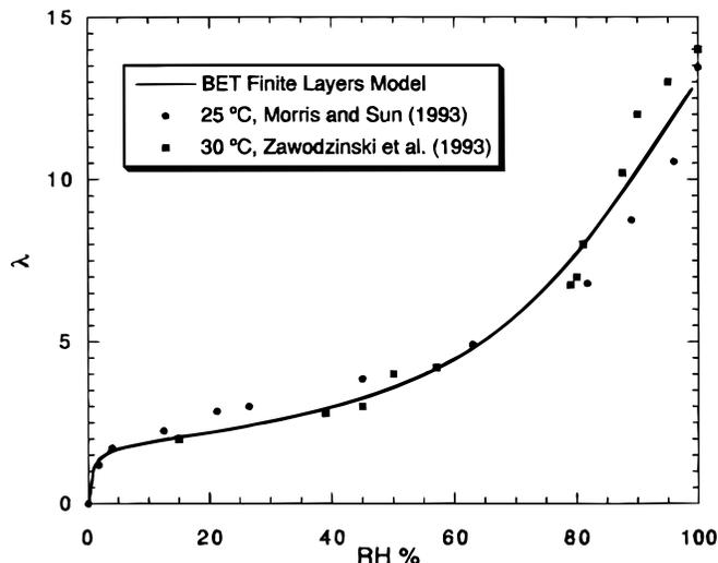
**Figure 2.** Adsorption isotherm for water uptake by Nafion 117 from water vapor. The finite-layer BET isotherm is compared with the data of Zawodzinski *et al.*<sup>53</sup> at 30°C and that of Morris and Sun<sup>37</sup> at 25°C for the parameters listed in Table I.
