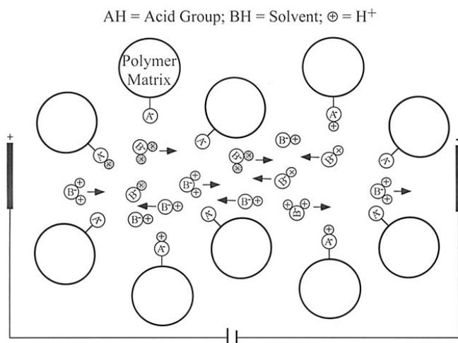
**Figure 1.** A “dusty-fluid model” depiction of a PEM. The polymer matrix along with an acid groups is viewed as “dust” particles comprising the PEM. The membrane imbibes a polar solvent BH (*e.g.*, HOH, CH<sub>3</sub>OH), that solvates the protons from the pendant acid HA forming BH<sub>2</sub><sup>+</sup> that serves as the charge carrier.
