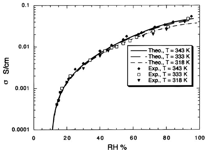
**Figure 5.** The experimental results of Sone *et al.*<sup>35</sup> for  $\sigma$  of Nafion 117 equilibrated in water vapor vs. RH or water vapor activity at different temperatures along with theoretical predictions for parameters listed in Table I.
