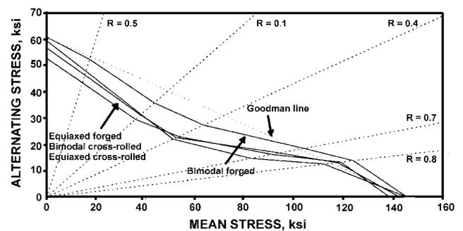
Fig. 2 Constant life diagrams at  $10^7$  cycles<sup>[11]</sup>
