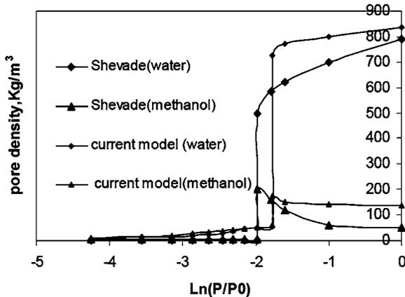
FIG. 17. Comparison of simulated pore densities of methanol and water with the results of Shevade *et al.* (big symbols) as a function of relative pressure for 20 Å pore size at  $y_{b1}=0.5$  (methanol) and 298 K.
