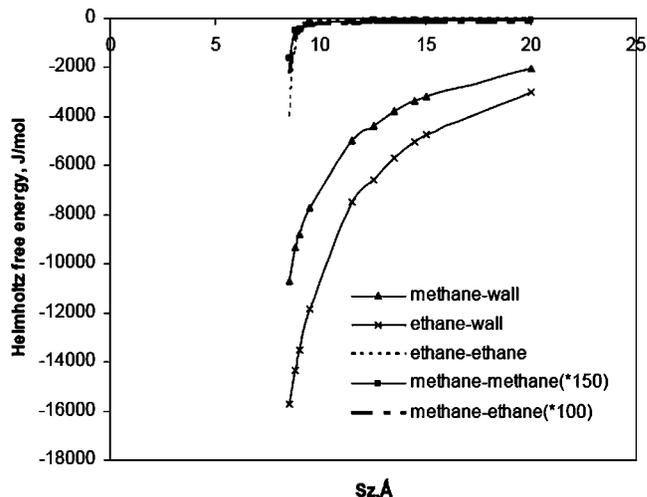
FIG. 2. Relative magnitudes of methane-wall, ethane-wall, ethane-ethane, methane-methane ( $\times 150$ ), and methane-ethane ( $\times 100$ ) interactions as a function of pore width for  $y_{b1}=0.9$  (methane) at 280 K.
