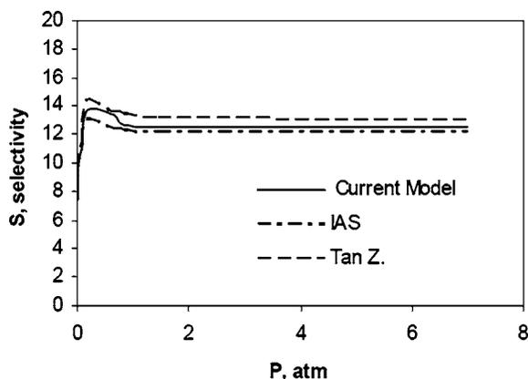
FIG. 9. Comparison of simulated ethane selectivity as a function of operating pressure with the results of Tan *et al.* (Refs. 5 and 6) and results from IAST for pore width of 9.7 Å at  $y_{b1}=0.9$  (methane) and  $T=286$  K.
