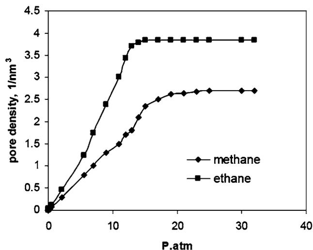
FIG. 8. Pore densities of methane and ethane as a function of operating pressure for 9.7 Å pore width at 286 K.
