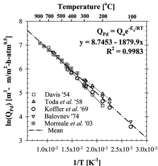
**Fig. 2** The Arrhenius plot of the literature data listed in Table 3 for the estimation of an average H<sub>2</sub> permeability for Pd foils.
