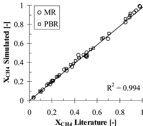
**Fig. 4** Literature *versus* simulated total methane conversion values.
