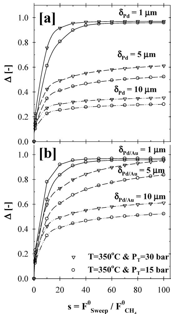
**Fig. 9** The effect of sweep gas flow rate on the (a) Pd- and (b) Pd/Au-based CMR performance ( $\text{H}_2\text{O}:\text{CH}_4:\text{He}_{\text{Sweep}} = 3:1:(1:10:100)$ ;  $T = 350\text{ }^\circ\text{C}$ ;  $P_T = 15\text{--}30\text{ bar}$ ;  $P_p = 1\text{ bar}$ ;  $r_0 = 2.5 \times 10^{-2}\text{ m}$ ;  $R_i = 6.6 \times 10^{-2}\text{ m}$ ;  $L = 12\text{ m}$ ;  $\delta_{\text{Pd}}$  or  $\text{Pd/Au} = 1\text{--}10\text{ }\mu\text{m}$ ;  $\phi_b = 0.50$ ;  $\eta = 1$ ).
