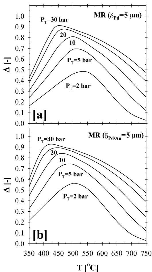
**Fig. 6**  $\Delta$ -index plot summarizing the impact of pressure and temperature effects on the total methane conversion for the (a) Pd- and (b) Pd/Au-based CMRs ( $\text{H}_2\text{O}:\text{CH}_4:\text{He}_{\text{Sweep}} = 3:1:10$ ;  $T = 350\text{--}750$  °C;  $P_T = 2\text{--}30$  bar;  $P_p = 1$  bar;  $r_0 = 2.5 \times 10^{-2}$  m;  $R_i = 6.6 \times 10^{-2}$  m;  $L = 12$  m;  $\delta_{\text{Pd}}$  or  $\text{Pd/Au} = 5$   $\mu\text{m}$ ;  $\phi_b = 0.50$ ;  $\eta = 1$ ).
