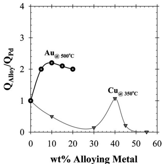
**Fig. 3** The normalized H<sub>2</sub> permeability plot for Pd, Pd/Au and Pd/Cu foils.<sup>2,48–50</sup>
