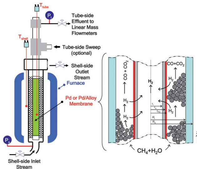
**Fig. 1** Schematic for the catalytic membrane reactor.
