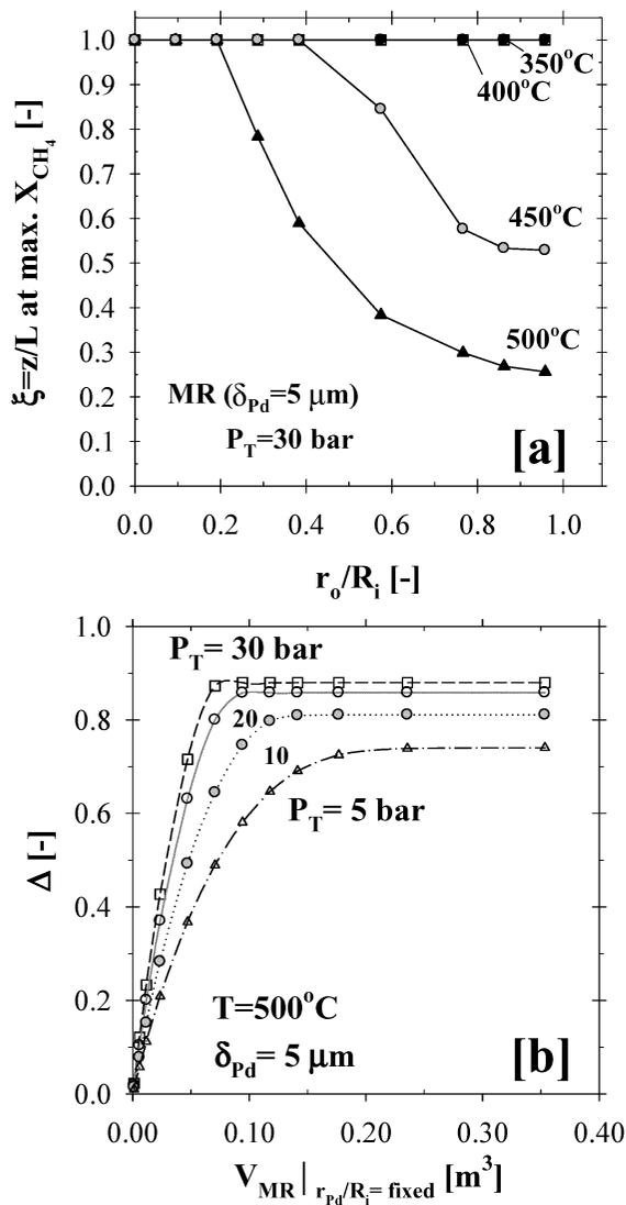
**Fig. 10** Reactor compactness and the effects of temperature and pressure on the (a) Membrane surface area ( $r_o/R_i$  ratio) and (b) Reactor volume ( $\text{H}_2\text{O}:\text{CH}_4:\text{He}_{\text{sweep}} = 3:1:10$ ;  $T = 350\text{--}500^\circ\text{C}$ ;  $P_T = 30$  bar;  $P_p = 1$  bar;  $r_o = 2.5 \times 10^{-2}$  m;  $R_i = 6.6 \times 10^{-2}$  m;  $L = 12$  m;  $\delta_{\text{Pd}} = 5 \mu\text{m}$ ;  $\phi_b = 0.50$ ;  $\eta = 1$ ).
