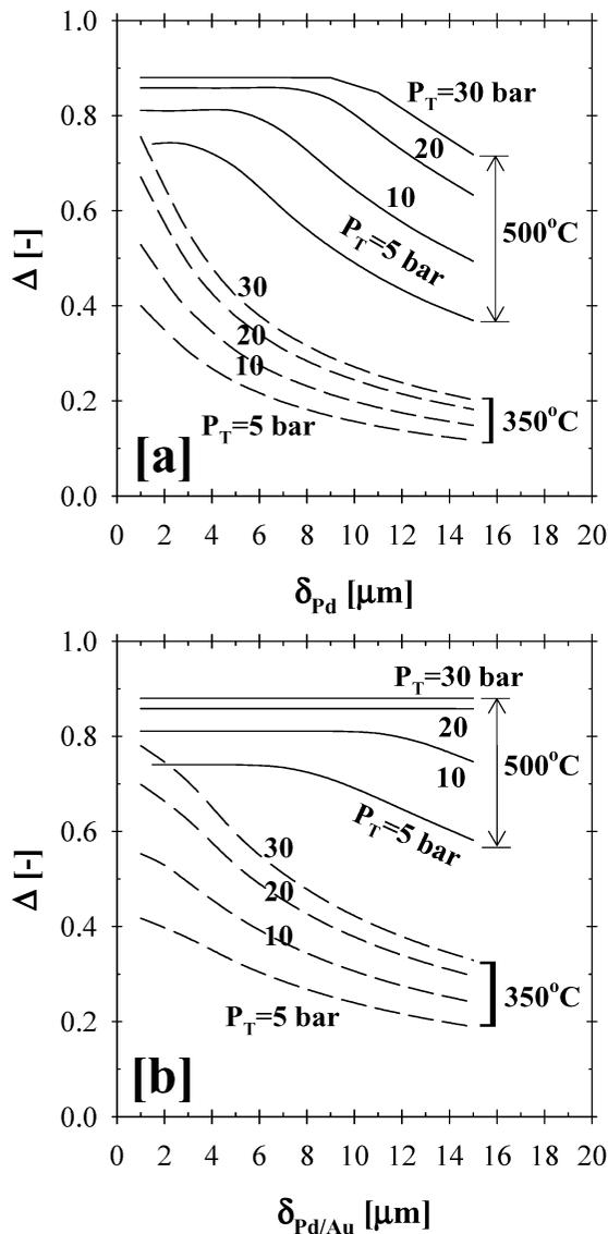
**Fig. 8** The effect of membrane thickness on the (a) Pd- and (b) Pd/Au-based CMR performance ( $\text{H}_2\text{O}:\text{CH}_4:\text{He}_{\text{Sweep}} = 3:1:10$ ;  $T = 350\text{--}500\text{ }^\circ\text{C}$ ;  $P_T = 5\text{--}30\text{ bar}$ ;  $P_p = 1\text{ bar}$ ;  $r_0 = 2.5 \times 10^{-2}\text{ m}$ ;  $R_i = 6.6 \times 10^{-2}\text{ m}$ ;  $L = 12\text{ m}$ ;  $\delta_{\text{Pd}}$  or  $\text{Pd/Au} = 1\text{--}15\text{ }\mu\text{m}$ ;  $\phi_b = 0.50$ ;  $\eta = 1$ ).
