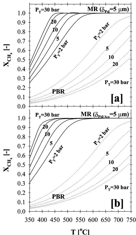
**Fig. 5** Temperature and pressure effects on the total methane conversion in (a) Pd- and (b) Pd/Au-based CMR and PBR ( $H_2O:CH_4:He_{Sweep} = 3:1:10$ ;  $T = 350-750$  °C;  $P_T = 2-30$  bar;  $P_P = 1$  bar;  $r_o = 2.5 \times 10^{-2}$  m;  $R_i = 6.6 \times 10^{-2}$  m;  $L = 12$  m;  $\delta_{Pd}$  or  $\delta_{Pd/Au} = 5$  μm;  $\phi_b = 0.50$ ;  $\eta = 1$ ).
