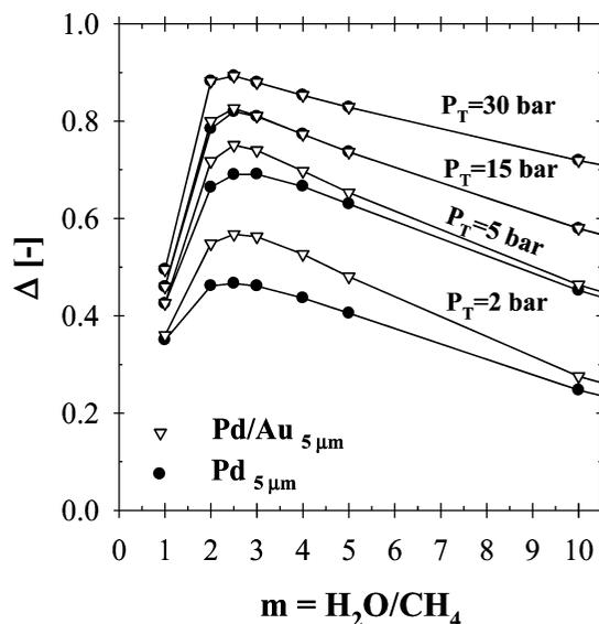
**Fig. 7** The effect of steam to methane ratio on CMR performance ( $\text{H}_2\text{O}:\text{CH}_4:\text{He}_{\text{Sweep}} = (1\text{--}10):1:10$ ;  $T = 500$  °C;  $P_T = 2\text{--}30$  bar;  $P_p = 1$  bar;  $r_0 = 2.5 \times 10^{-2}$  m;  $R_i = 6.6 \times 10^{-2}$  m;  $L = 12$  m;  $\delta_{\text{Pd}}$  or  $\text{Pd/Au} = 5$   $\mu\text{m}$ ;  $\phi_b = 0.50$ ;  $\eta = 1$ ).
