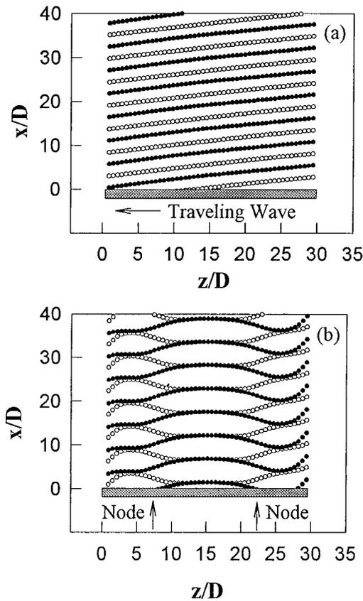
FIG. 8. Oblique shedding patterns for traveling wave along cable span. (a) Traveling wave case, (b) standing wave case.  $\Omega = 1.0$ ,  $K_n = 0.01$ ,  $k^* = 100$ ,  $k_{\text{wave}} = 100$ ,  $A/D = 0.68$  at antinode,  $Re = 100$ ,  $U_c/U_\infty = 0.88$ , periodic boundary conditions,  $\beta = 10^\circ$ ,  $AR = (U_c/U_\infty)/(St \tan \beta) = 30$ .
