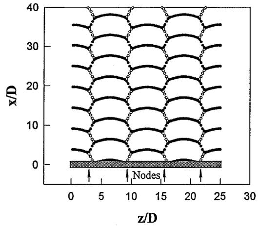
FIG. 7. Honeycomblike wake structure for higher-order mode shape at large forcing amplitude.  $\Omega=1.0$ ,  $K_0=1.2$ ,  $k^*=100$ ,  $k_{wave}=50$ ,  $A/D=0.68$  at antinode,  $AR=25$ ,  $Re=100$ ,  $U_c/U_\infty=0.88$ , periodic-free boundary conditions. Simultaneous shedding occurs near cable anti-nodes.
