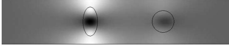
Figure 6: Eigenfunction for the third real eigenvalue  $\epsilon_1 \approx 11.42$  for the parameters  $\omega = 0.3, \epsilon_0 = 1, \mu_0 = 1, \mu_1 = 3, \kappa_1 = 0.4$ . This is a robust guided mode.
