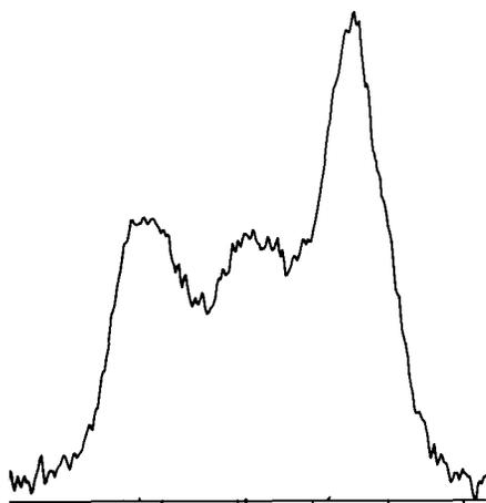
FIG. 1. Experimental x-ray intensity vs  $2\theta$  for the (400) cubic and (400), (004) tetragonal peaks.
