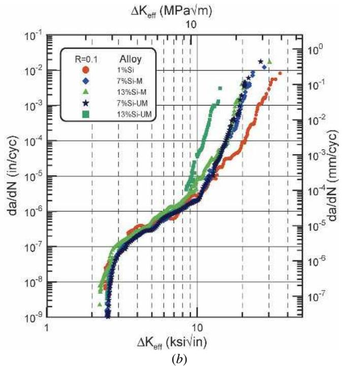
Fig. 14—The FCG data for all alloys after closure correction: (a) HRS and (b) LRS.
