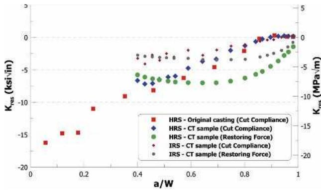
Fig. 12—Variation of  $K_{res}$  with crack length for HRS and IRS samples.
