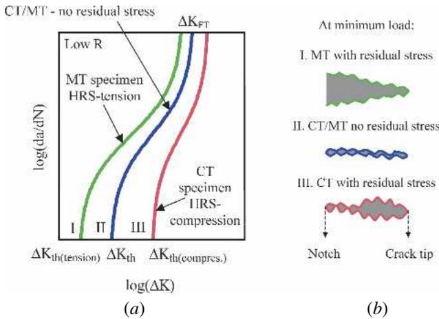
Fig. 5—The effects of compressive (CT specimen) and tensile (MT specimen) residual stresses on: (a) FCG behavior and (b) crack behavior at minimum load.
