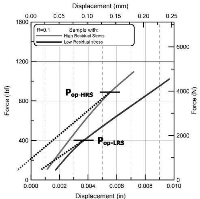
Fig. 2—Load-displacement records showing microstructure/roughness-induced closure (right curve) and the additional effect of residual stress on crack closure level (left curve). The  $P_{op}$  is the force required to fully open the crack under HRS and LRS conditions.
