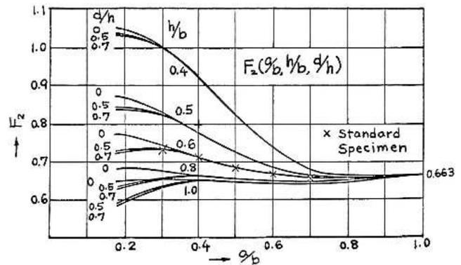
Fig. 10—Variation of  $F_2$  parameter as a function of the specimen geometry.<sup>[29]</sup>
