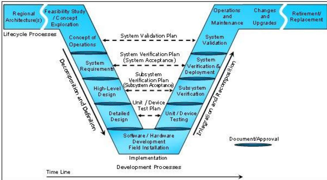
Figure 1. The systems engineering “V” model, depicting the systems engineering life cycle (Federal Highway Administration, 2013).
