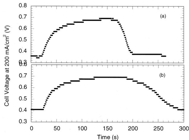
**Figure 3.** Recovery and poisoning transient for the cell operated at  $200 \text{ mA}/\text{cm}^2$  at  $80^\circ\text{C}$  for different anode inlet flow rates. (a) 80 and (b) 57.5 sccm. Nafion 115 membrane.
