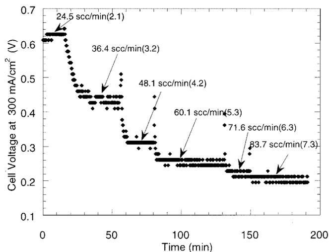
**Figure 2.** Cell voltage profile at different anode inlet flow rates at  $300 \text{ mA}/\text{cm}^2$  at  $80^\circ\text{C}$ ; Nafion 115 membrane. Numbers in parentheses are the corresponding stoichiometry.
