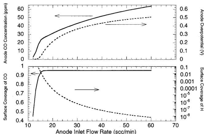
**Figure 10.** Model prediction of the steady-state CO and H surface coverage, CO content in anode chamber and the anode overpotential as a function of anode inlet flow rate at 80°C and 200 mA/cm<sup>2</sup>; model parameters have values given in Table I.
