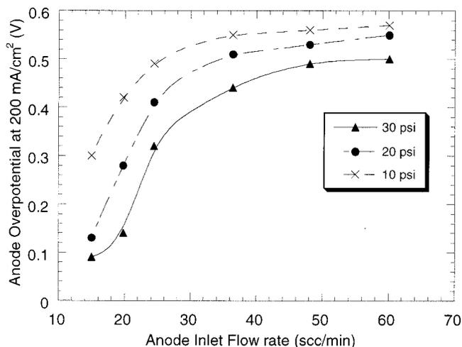
**Figure 7.** Anode overpotential vs. flow rate at 200 mA/cm<sup>2</sup> at different cathode O<sub>2</sub> pressures; 80°C; Nafion 115 membrane.
