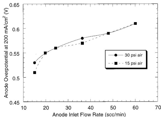
**Figure 9.** Anode overpotential vs. flow rate at 200 mA/cm<sup>2</sup> at different cathode air pressures; 80°C; Nafion 115 membrane.
