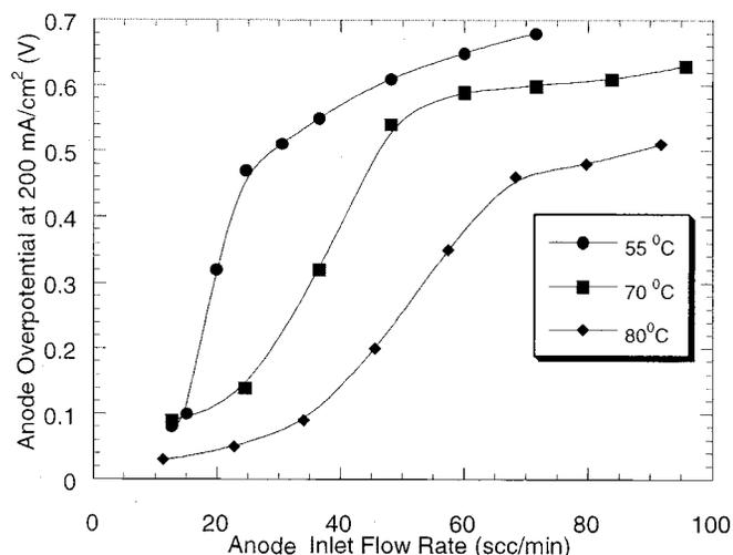
**Figure 6.** Anode overpotential vs. flow rate at 200 mA/cm<sup>2</sup> at different temperatures; Nafion 115 membrane.
