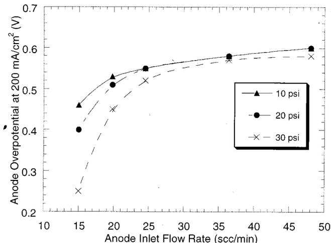
**Figure 8.** Anode overpotential vs. flow rate at 200 mA/cm<sup>2</sup> at different cathode O<sub>2</sub> pressures; 80°C; Nafion 117 membrane.
