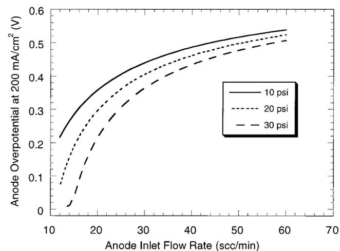
**Figure 12.** Model calculations of the steady-state anode overpotential as a function of anode inlet flow rate for different cathode O<sub>2</sub> pressures at 80°C and 200 mA/cm<sup>2</sup>. Model parameter values are given in Table I.
