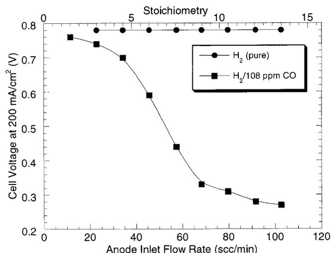
**Figure 1.** Effect of anode flow rate on cell voltage at constant current density for  $\text{H}_2$  and  $\text{H}_2/108$  ppm CO for  $5 \text{ cm}^2$  PEM fuel cell at  $80^\circ\text{C}$ ; Nafion 115 membrane. Current density,  $200 \text{ mA}/\text{cm}^2$ .
