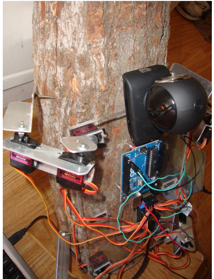
Figure 4. The robot gripping a tree log using the spike type legs.
