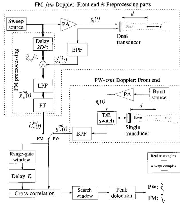
FIG. 2. Block diagram of PW-tsm and FM-fsm signal processing. With the actual switch setting, the system functions as a PW-tsm Doppler system.  $\hat{\tau}_p$  and  $\hat{\gamma}_p$  denote the estimated location of the global peak of the cross-correlation function, within the search window, from which the velocity is estimated.
