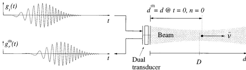
FIG. 1. Sketch of idealized measurement situation. A single scatterer is moving with velocity,  $v$ , axially along the axis of the transmitted beam in the direction away from the transducer. It is located at range  $d^{(0)}$  at  $t=0$  and  $n=0$ . The nominal range,  $D$ , will be introduced in Sec. III. To the left, one transmitted signal with the corresponding received signal is shown.
