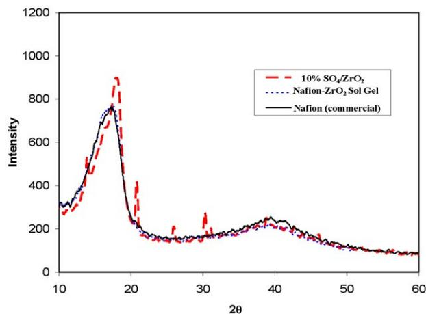
**Figure 7.** XRD pattern for composite membranes and Nafion.
