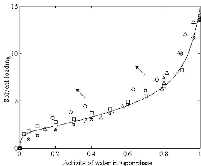
**Figure 3.** The solvent loading vs. activity of water vapor for Nafion (EW = 1100) membrane (triangle: Ref. 20, square: Ref. 21, circle: Ref. 44, and star: This work). The design objective is to increase the solvent loading of Nafion. The composite will adsorb more water at fixed RH vs. unmodified Nafion resulting in higher conductivity at low RH.
