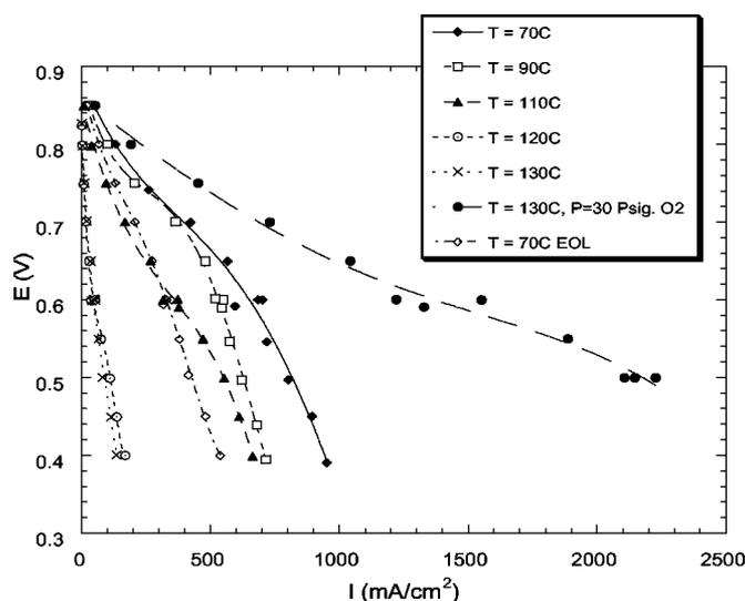
**Figure 10.** The cell performance of Nafion 112 MEA with conditions as noted on figure. Operated with 1.5 atm air/H<sub>2</sub>, humidifiers set at 80°C. The exception was when the cell was at 130°C, 3 atm. O<sub>2</sub> and the humidifiers set at 130°C.
