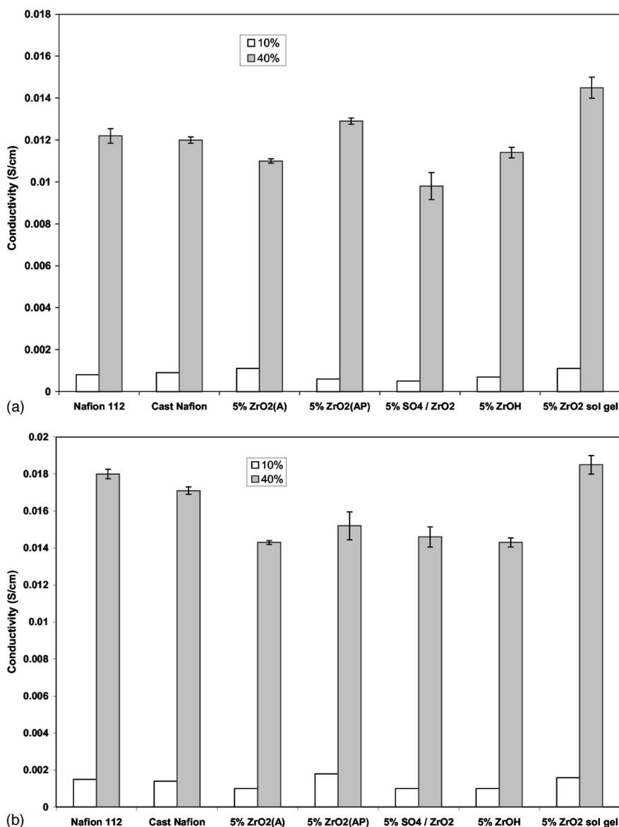
**Figure 8.** (a, top) The conductivity of the PEMs at 10% RH and 40% RH at 90°C. The Nafion ZrO<sub>2</sub> sol-gel PEM shows the highest conductivity of the samples. (b, bottom) The conductivity of the PEMs at 10 and 40% RH at 120°C. The Nafion ZrO<sub>2</sub> sol-gel PEM shows the highest conductivity of the samples.
