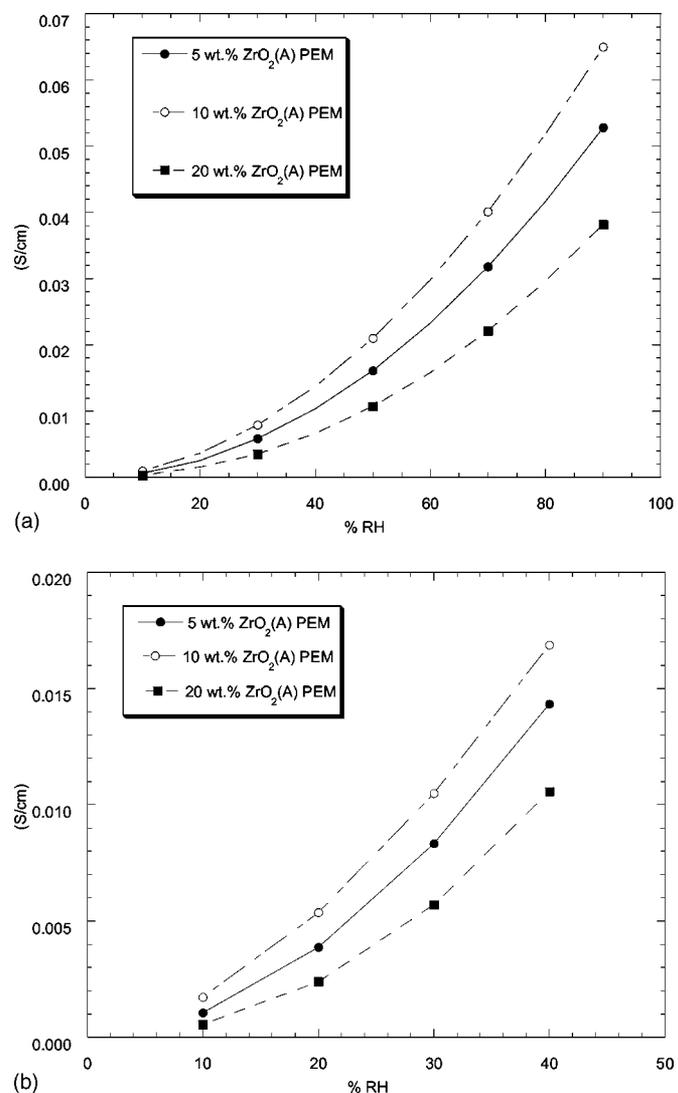
**Figure 9.** (a, top) The conductivity of loaded composite PEMs at 90°C vs. RH. The optimum conductivity is observed with the 10 wt % PEM. (b, bottom) The conductivity of loaded composite PEMs at 120°C. The optimum conductivity is observed with the 10 wt % PEM.
