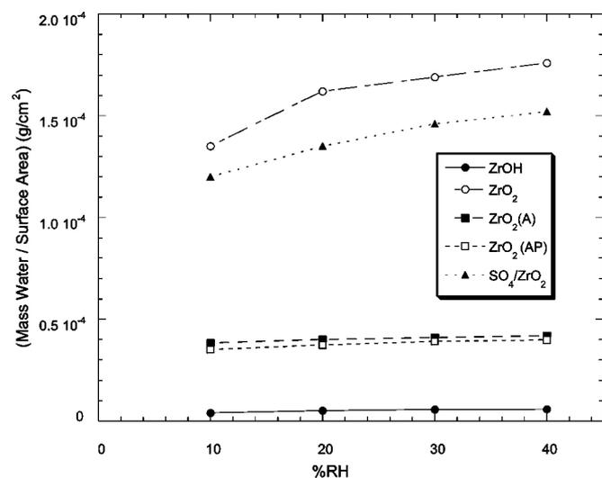
**Figure 5.** The surface area normalized water uptake of the powder at 120°C vs. RH. The most promising candidates are the ZrO<sub>2</sub> and the SO<sub>4</sub>/ZrO<sub>2</sub> samples.
