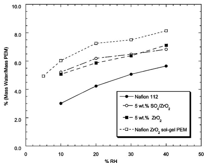
**Figure 6.** The water uptake of composite membranes and Nafion 112 at 120°C vs. RH. The Nafion ZrO<sub>2</sub> sol-gel PEM demonstrates the highest water uptake.
