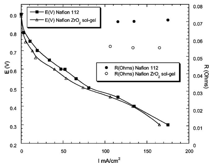
**Figure 11.** The cell performance of Nafion 112 MEA vs. Nafion ZrO<sub>2</sub> sol-gel composite MEA. Air and H<sub>2</sub> at 2.0 and 1.3 times stoichiometry flows, respectively,  $P = 1.0$  atm.,  $T_{\text{humidifier}} = 80^\circ\text{C}$ ,  $T_{\text{cell}} = 110^\circ\text{C}$ .
