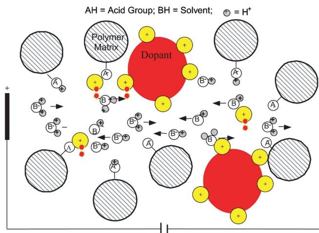
**Figure 2.** A dusty-fluid model depiction of a PEM describing proton conductivity through the Nafion polymer matrix and the superacidic dopant. The framework treats the Nafion matrix as large dust particles through which the current carrying ions must traverse.
