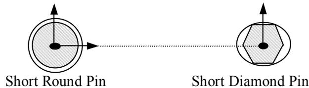
**Figure 5.4 Locating Points for Pin-Hole Locating**
