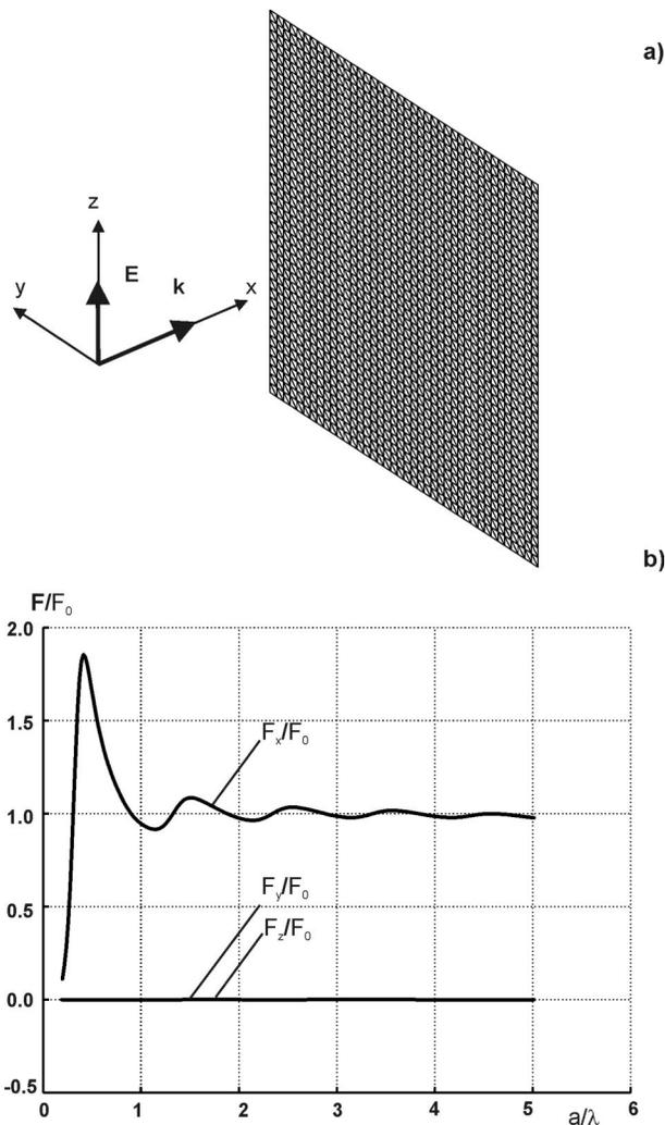
FIG. 1. (a) Geometry of incident signal for the single plate and (b) net radiation force as a function of the plate size/wavelength ratio. The original (simulation) plate mesh had  $60 \times 60$  rectangles (10 680 unknowns); 250 frequency steps are employed to cover the entire domain of  $a/\lambda$ .
