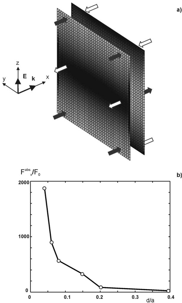
FIG. 3. (a) Force density distribution for the parallel-plate resonator with  $d/a=0.15$  at the first resonance. The surface gray scale extends from black (maximum force density in the direction of the negative  $x$  axis) to white (maximum force density in the direction of the positive  $x$  axis) and (b) magnitude of the force density integrated over the surface area  $F_x^{\text{abs}}$  for different ratios of  $d/a$  at the first resonance.
