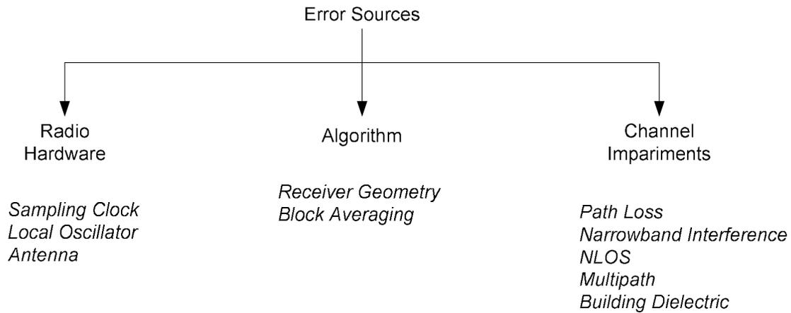
**Figure 6 Types of Error Sources.**
