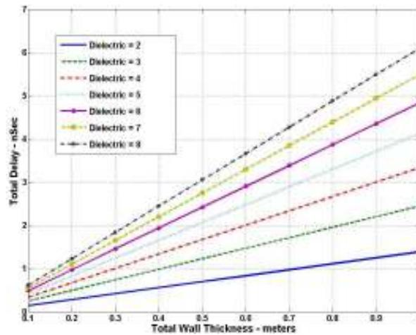
**Figure 10 Wall Thickness vs. Signal Delay for Various Dielectric Constants**
