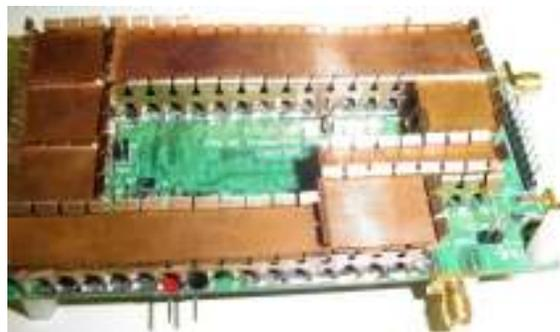
**Figure 4 RF Transmitter Front End PCB**
