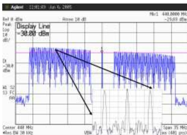
**Figure 2: MC-UWB Signal Structure**
