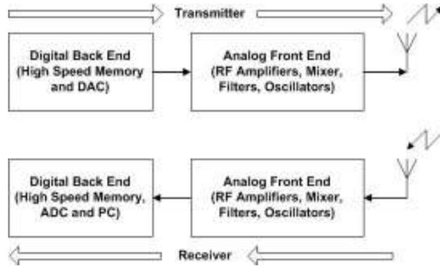
**Figure 3: Overview of the RF Prototype System Architecture**
