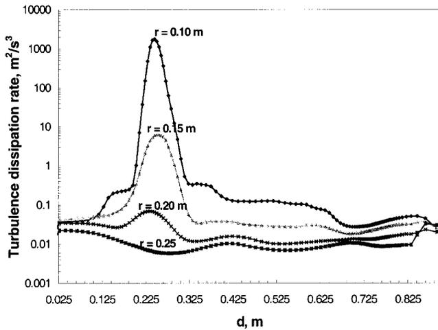
Fig. 8—Turbulence dissipation rate as a function of the distance from the furnace bottom ( $d$ ) and radial distance from the center of the furnace ( $r$ ) for a conventional flotation reactor at  $t = 420$  s, 675 rpm rotation speed, and 36 L/min gas flow rate.
