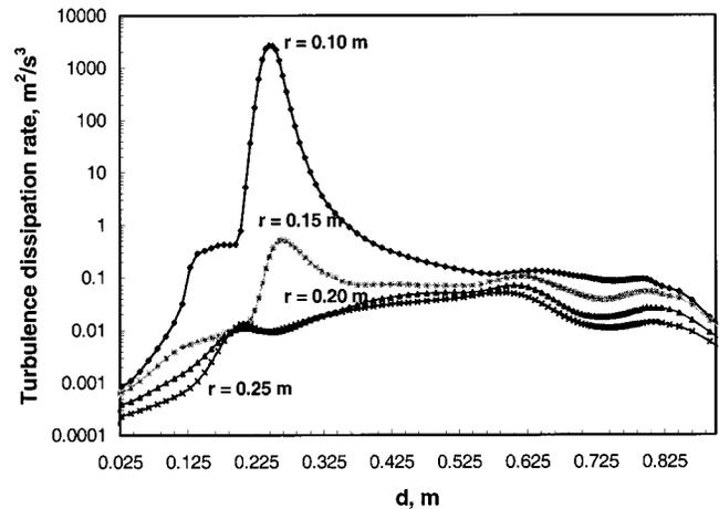
Fig. 9—Turbulence dissipation rate as a function of the distance from the furnace bottom ( $d$ ) and radial distance from the center of the furnace ( $r$ ) of a reverse rotation flotation reactor at  $t = 420$  s, rotation 675 rpm, and gas flow rate 36 L/min.
