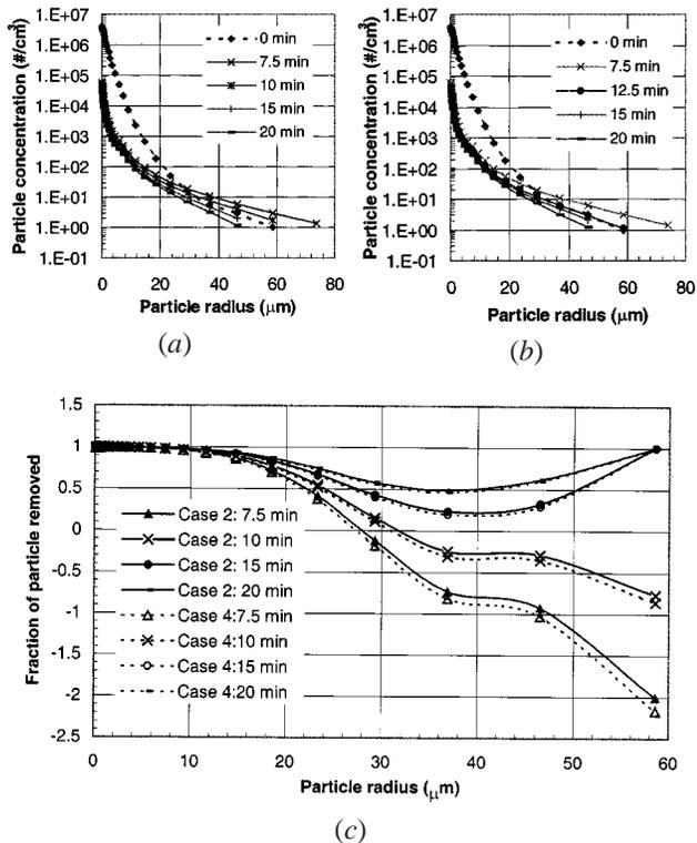
Fig. 12—Effects of gas flow rate on particle size distribution in a rotary degasser. (a) Particle concentration profile for case 2, (b) profile for case 4, and (c) particle removal efficiency.
