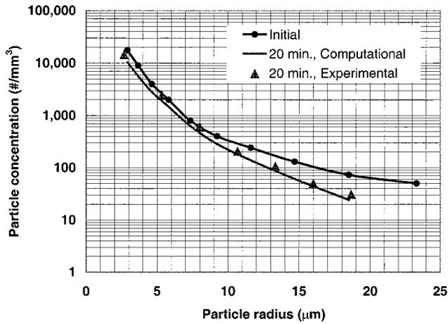
Fig. 8—Comparison between measured and model predicted particle concentration vs particle radius curves.
