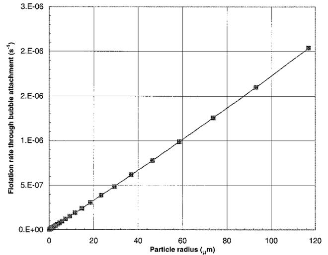
Fig. 6—Variation of the flotation rate due to bubble attachment with particle size.
