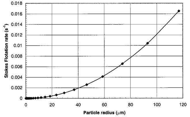
Fig. 3—Variation of Stokes flotation rate with particle size in a typical rotary degasser.
