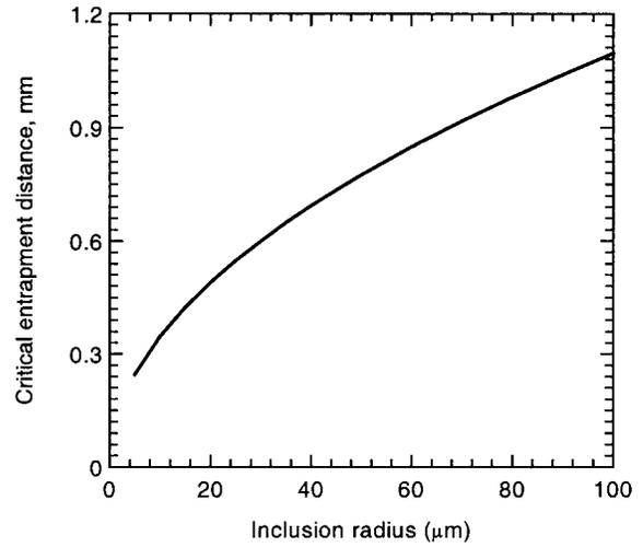
Fig. 5—Critical entrainment distance as a function of particle radius.
