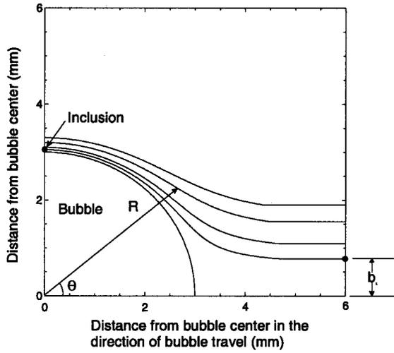
Fig. 4—Streamlines around a 6 mm diameter argon gas bubble based on the assumption of potential flow.
