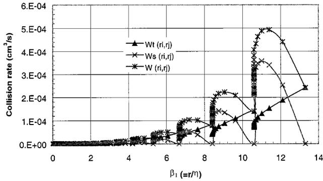
Fig. 2—Variation of particle collision rate with particle size in a rotary degasser operating at 675 rpm with a gas flow rate of 36 L of argon per minute.
