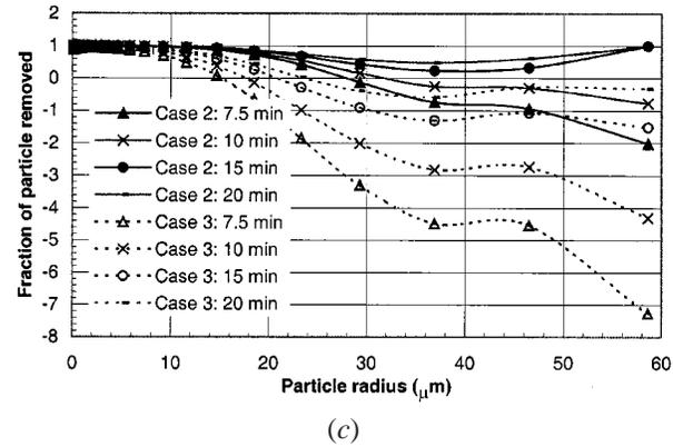
Fig. 10—Effect of rotation direction on particle size distribution in a rotary degasser. (a) Particle concentration profile for case 1, (b) particle concentration profile for case 2, and (c) particle removal efficiency.
