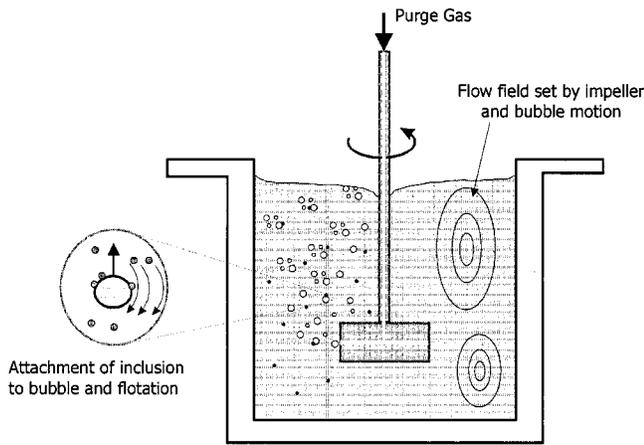
Fig. 1—Flotation treatment process using a rotary degasser.
