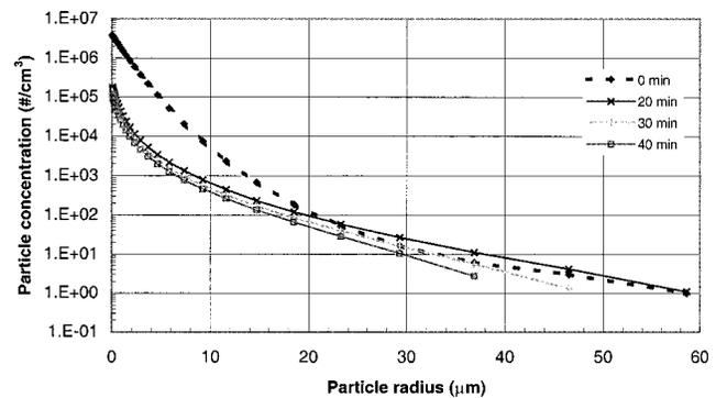
Fig. 9—Particle size distribution in a rotary degasser operating at 350 rpm, 36 L/min gas flow rate and periodic reversal of rotation direction.
