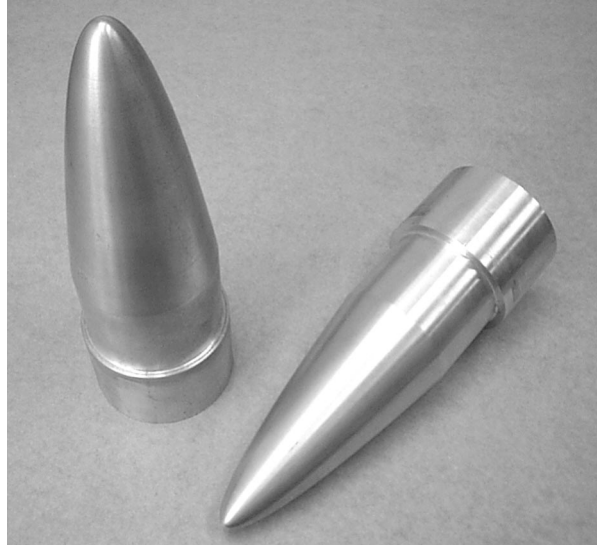
Fig. 7 Two samples of the paraboloid-of-revolution model. The pieces are 229.0 mm in height with a cylindrical base diameter of 76.12 \pm 0.040 mm (as measured with conventional contact techniques). The parabolic section of one of the pieces is to be measured using the OEH method.
