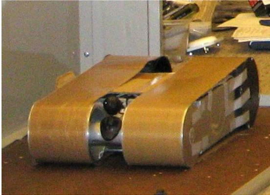
Prototype 2 with the wheels taped so they can not move. This was done for a friction test of the belts.
