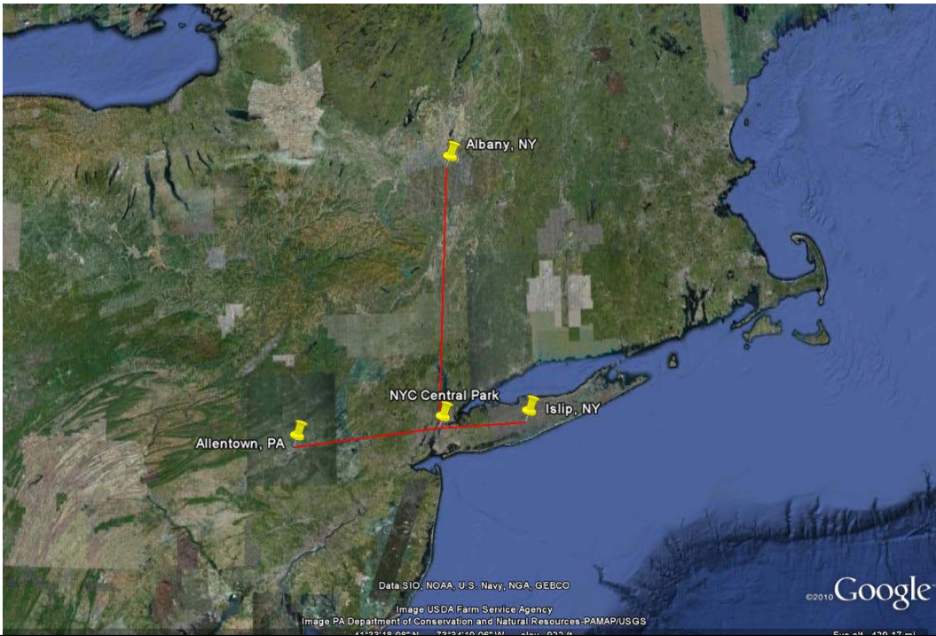
Figure 3: lines drawn between the weather stations analyzed in Table 1. Data found from calculating distance was used to calculate Cartesian coordinates of weather stations. Note that NYC Central Park is used as the origin. Source: Google Earth©
