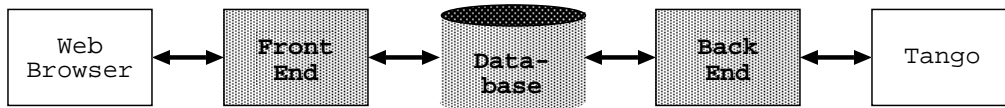
Figure 1: The P-Tango System Architecture. P-Tango consists of a front end, database and back end. The user accesses the front end through a web browser. The back end downloads articles from the Worcester Telegram and Gazette Online (Tango).
