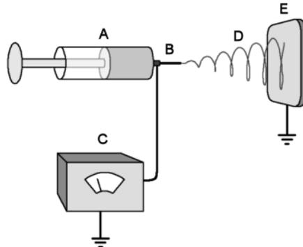
*Figure 3: Process of Electrospinning (Ramakrishna, et al., 2005)*
