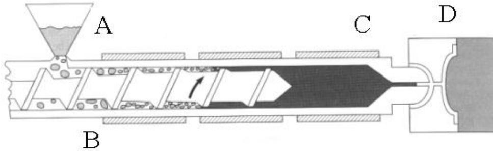
Figure 4: Process of Injection Molding (Strong, 2000)
