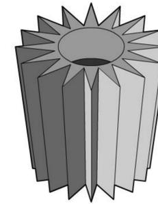
Unlike the first design, a Peltier cooler would be attached directly to the inside of a large piece of metal with maximized surface area (left). The cold metal would condense water out of the air which would then drip down, pass through a charcoal filter and be collected into a large storage container.
