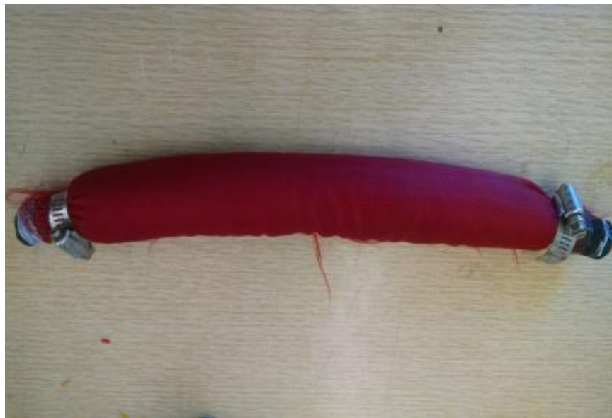
Figure 5: 1 st Generation HydroBone utilizing granulated EPDM rubber
