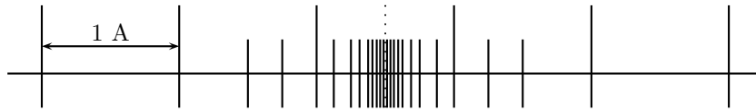
Figure 10.4: Detailed structure of the non-uniform grid at the well-barrier interface. Grid steps of 1, 0.5, 0.25, 0.125, 0.0625, 0.03125, and 0.025 Å are used.
