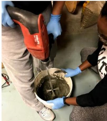
*Figure 7: New mixing setup with a hand held electric drill and a mixing paddle*
