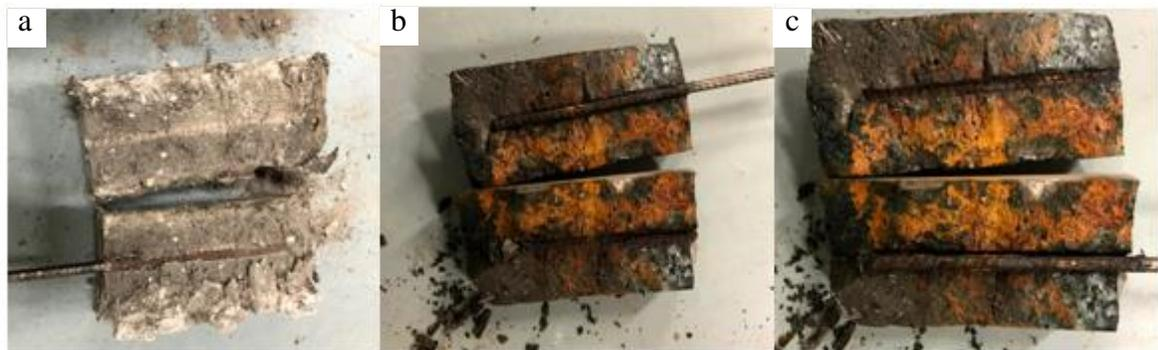
*Figure 16: Cross section of samples after corrosion testing showing that the rebar reinforced concrete sample with plastic fibers (a) did not corrode unlike the glass (b) and steel (c) samples*
