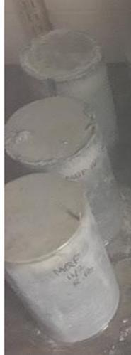
*Figure 5: Initial samples showing a watery and light grey substance that collected at the top*
