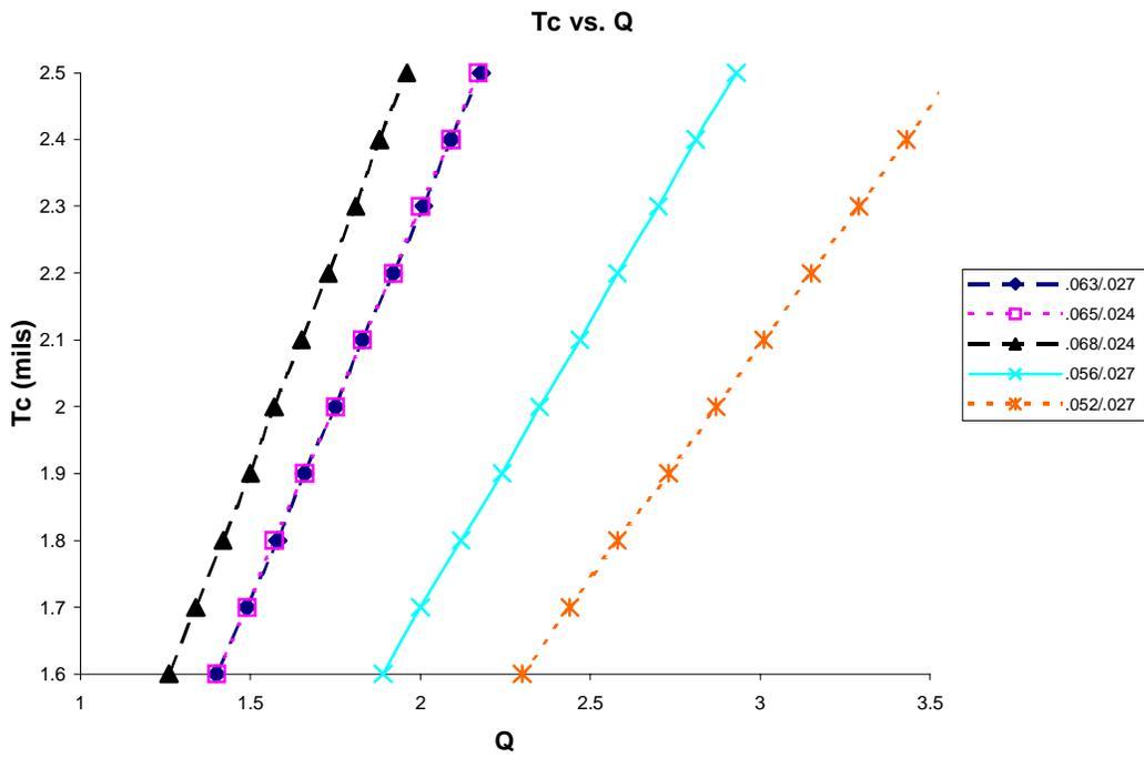
Figure 4.3 Double wall thickness of balloons ( $T_c$ ) versus the bottom number of their corresponding stretch ratio ( $Q$ ). Data were calculated for theoretical  $T_c$ s within the accepted 5mm balloon specification with tube dimensions previously used for twelve-layer tubes.
