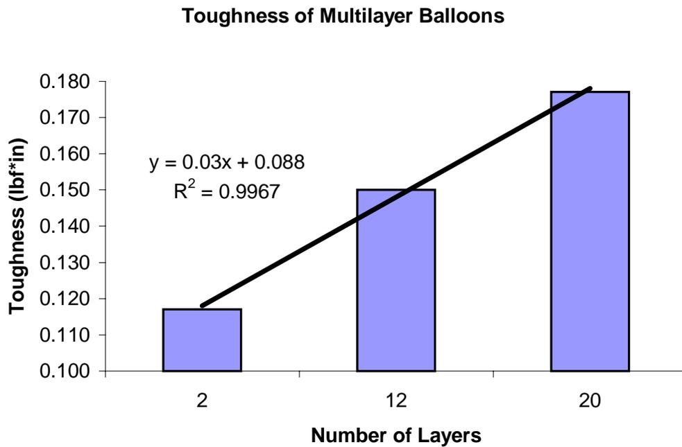
*Figure 4.6 Toughnesses of 5mm 80/20 PET/Hytrel<sup>®</sup> balloons with an increasing number of layers. Each value is the average of 10 balloons tested.*
