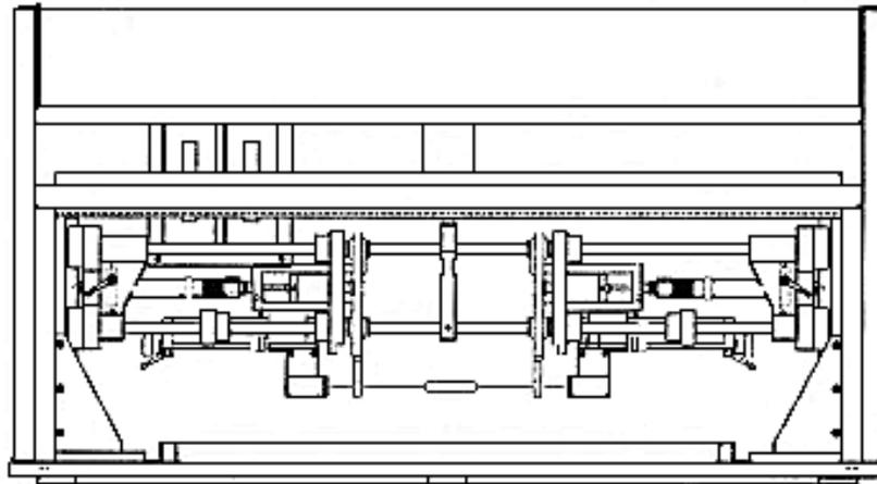
*Figure 2.10 A typical machine used to free-blow angioplasty balloons. The balloon has been blown from a tube threaded between two grippers that was lowered into a glycerin bath and pressurized.<sup>21</sup>*
