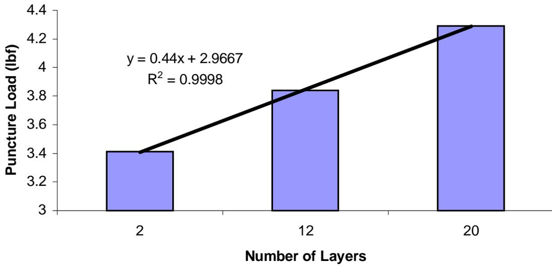
Figure 4.5 Puncture resistances of 5mm 80/20 PET/Hytrel<sup>®</sup> balloons with an increasing number of layers. Each value is the average of 10 balloons tested.
