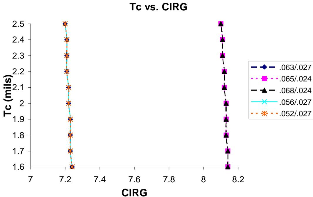
Figure 4.2 Double wall thickness of balloons (Tc) versus the top number of their corresponding stretch ratio (CIRG). Data were calculated for theoretical Tcs within the accepted 5mm balloon specification with tube dimensions previously used for twelve-layer tubes.
