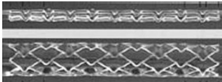
*Figure 2.2 A NIR<sup>®</sup> stent before (top) and after (bottom) expansion.<sup>3</sup>*
