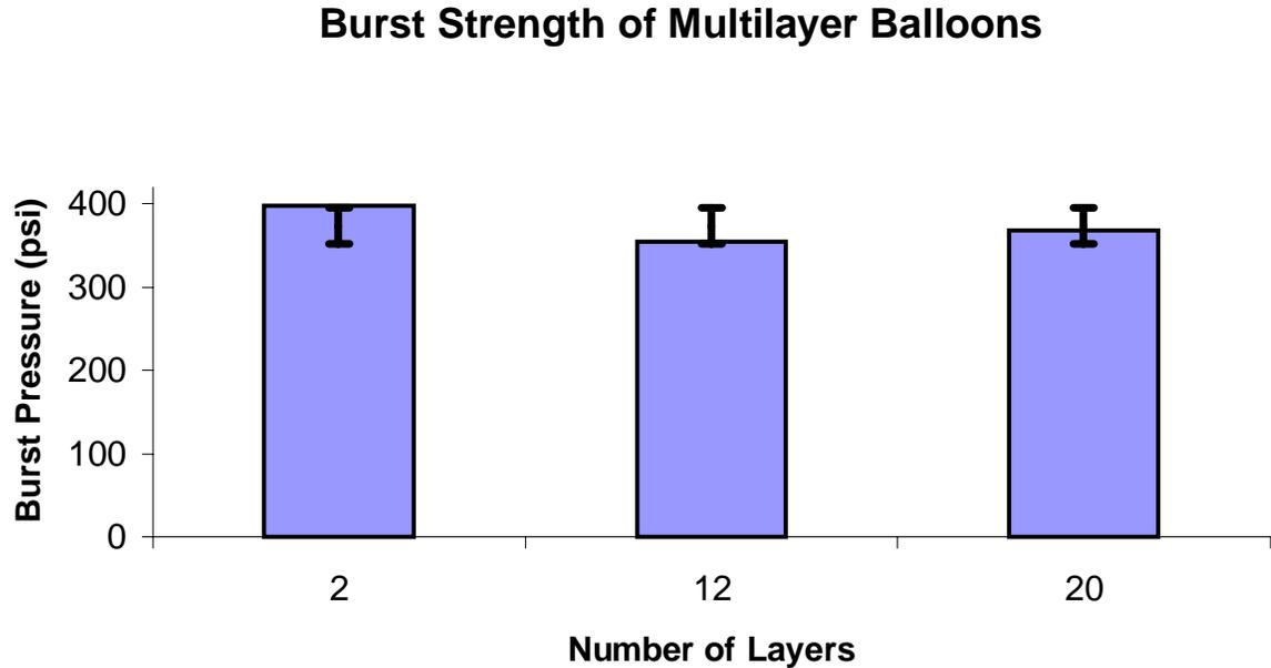
*Figure 4.4 Burst strengths of 5mm 80/20 PET/Hytrel<sup>®</sup> balloons with an increasing number of layers. Each value is the average of 10 balloons tested. Error bars signify one standard deviation.*
