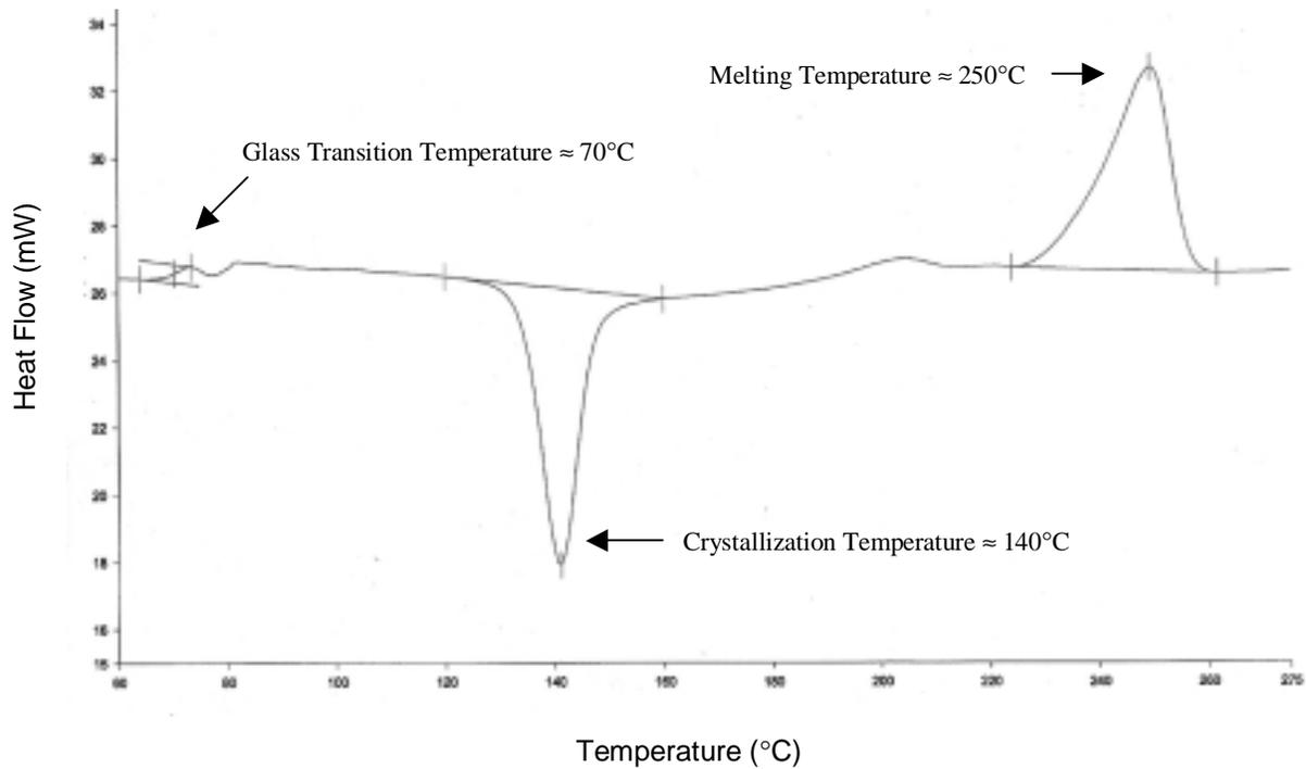
*Figure 2.11 A Differential Scanning Calorimeter plot of an 80/20 PET/Hytrel<sup>®</sup> extruded tube used in this investigation, with the PET transitions labeled. The tube was heated from 0 to 300 °C at 20 °C/min in a Perkin-Elmer DSC7.*
