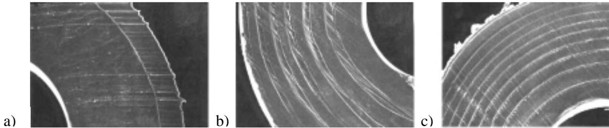
*Figure 3.0.2 SEM micrographs of cross-sections of a) two-layer, b) twelve-layer, and c) twenty-layer 80/20 PET/Hytrel<sup>®</sup> 5mm balloon tubes (150x)*
