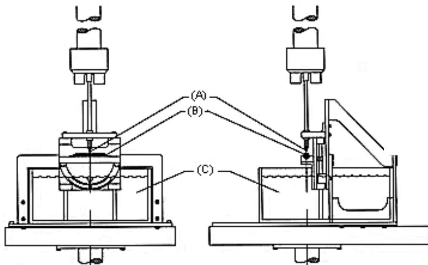
Figure 3.0.4 Fixture used with an Instron for puncture testing with (A) puncture tip, (B) balloon, and (C) heated water bath.<sup>37</sup>
