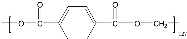
Figure 3.0.1 Chemical structure of Shell Cleartuf™ 8006
