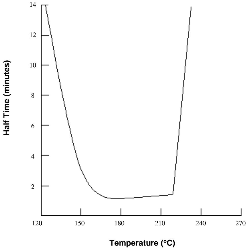
Figure 2.9 Half time crystallization rate versus temperature for PET.<sup>20</sup>
