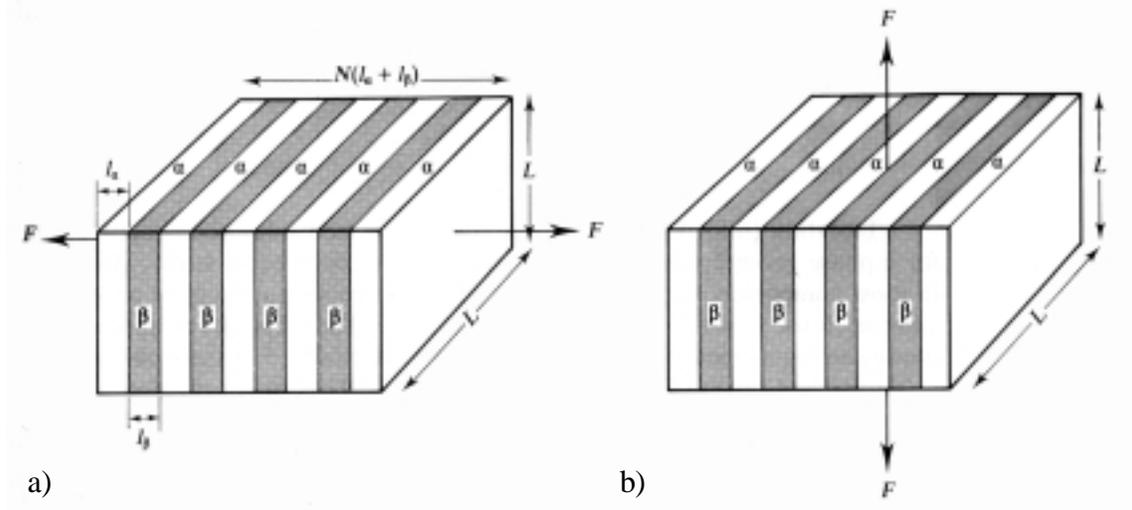
Figure 2.14 Composite structure having layers of two different materials ( $\alpha$  and  $\beta$ ). A tensile force ( $F$ ) is applied normal to the broad faces of the layers in a) and perpendicular to them in b).<sup>41</sup>
