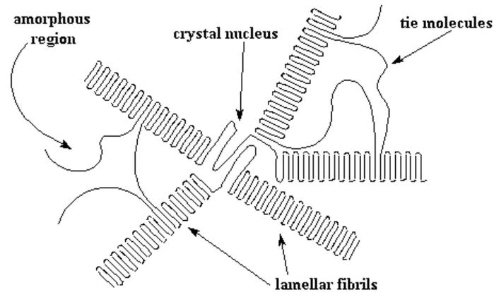
Figure 2.13 A polymeric spherulite composed of long molecules.<sup>31</sup>
