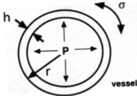
Figure 2.4 *Mechanics of balloon inflation in an atherosclerotic blood vessel. As pressure ( $P$ ) is applied inside the vessel, stress ( $\sigma$ ) is produced in the vessel wall in relation to the thickness of the plaque ( $h$ ) and the vessel radius ( $r$ ) such that  $\sigma = (Pr/h)$ .<sup>6</sup>*
