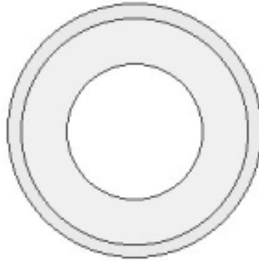
*Figure 2.7* Cross-section of an extruded tube used to fabricate a two-layered angioplasty balloon. The inner layer is PET, and the outer layer is Hytrel<sup>®</sup>.
