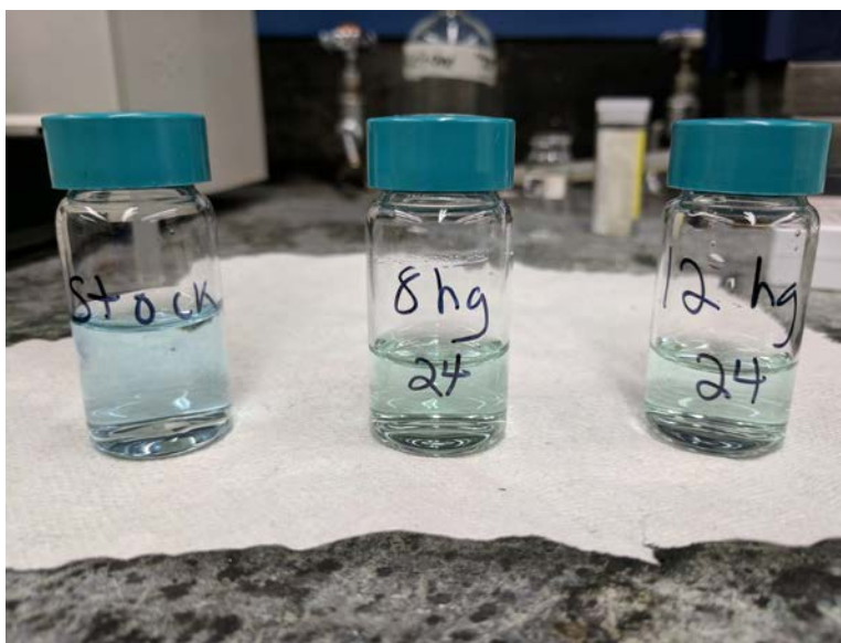
Figure 4: Comparing colors of filtered solutions of 8 and 12 hour glucose hydrochars
