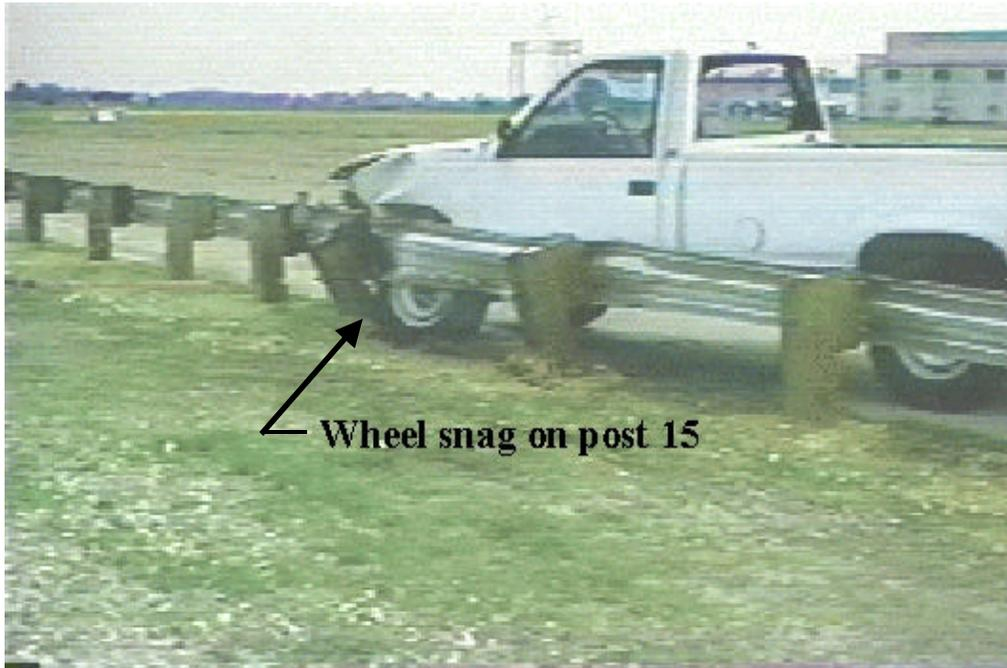
**Figure 1. Full scale test showing wheel snagging. (6)**
