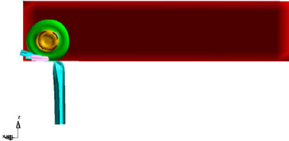
Figure 29. The steel W150x13.5 post assembled with the wheel with vehicle inertia.
