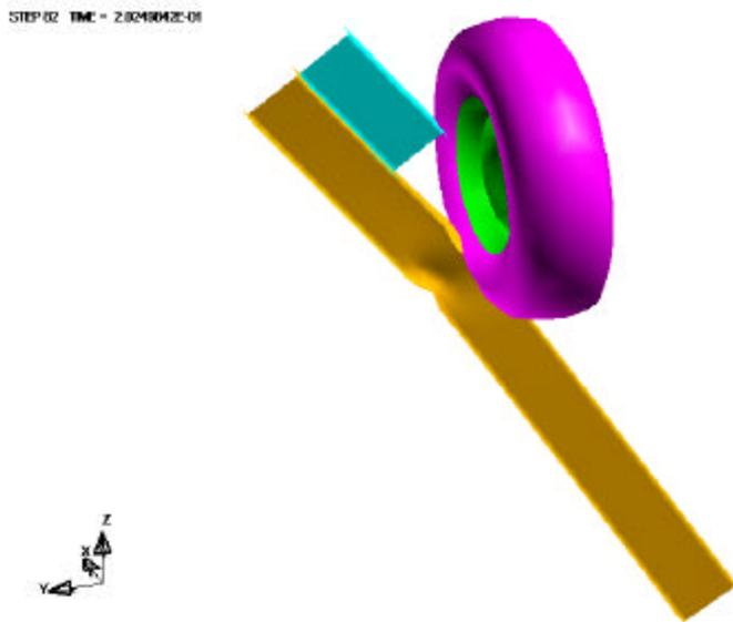
Figure 27. Steel post W150x23.5 and wheel that snag.
