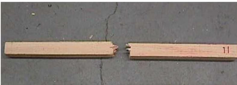
**Figure 6. Typical failure of the tested wood specimens.**
