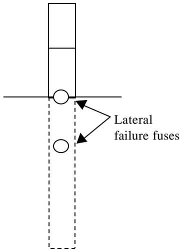
**Figure 34. Sketch showing post with lateral failure fuses.**
