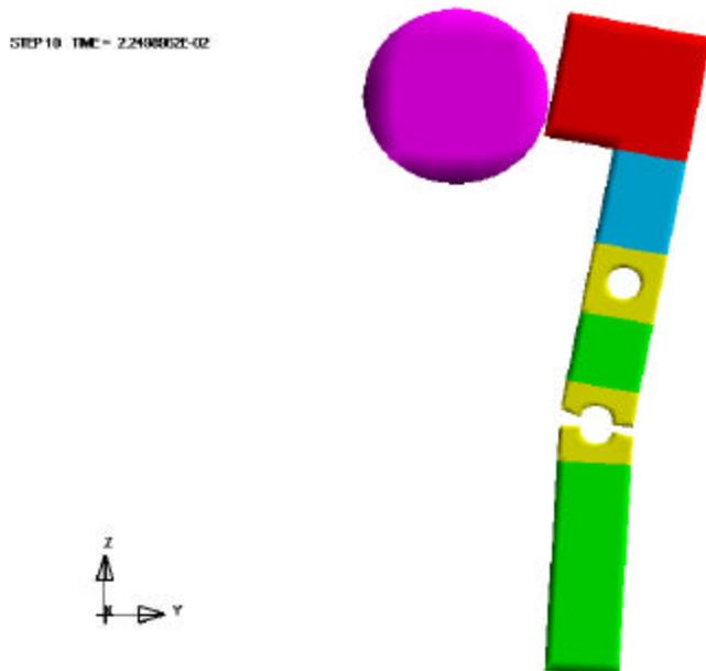
**Figure 46. CRT post failure caused by lateral loading.**
