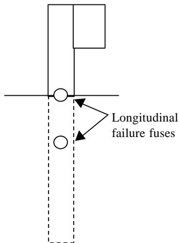
**Figure 33. Sketch showing post with longitudinal failure fuses.**
