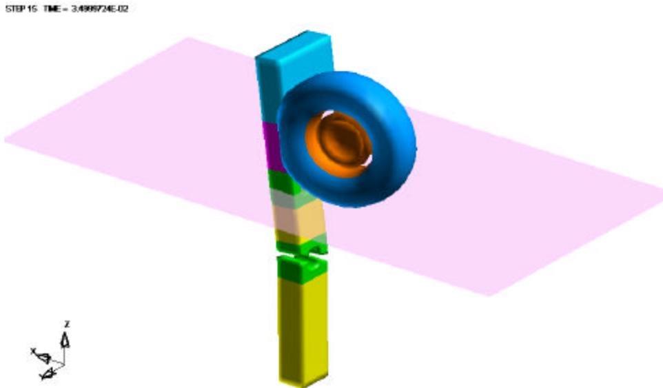
**Figure 50. CRT post failure caused by wheel impact.**
