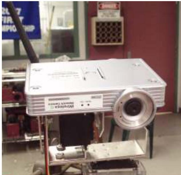
**Fig. 18. Camera Mounting Bracket**
