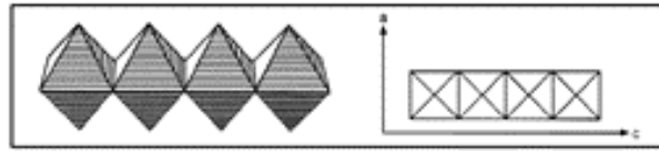
Figure 2. A diagram of the rutile crystal [15]
