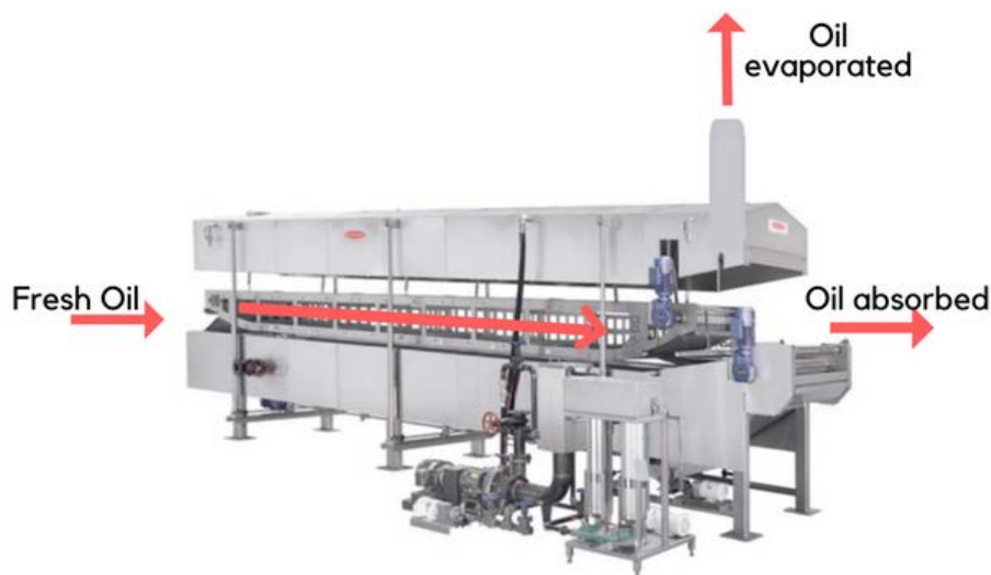
Figure 4: Chip Fryer Mass Balance
