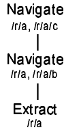
Figure 3.7: A top-down approach. The query plan is executed bottom-up. The bottom-most operator evaluates the root node of the binding tree, while the two consecutive navigate operators evaluate the two leaf nodes
