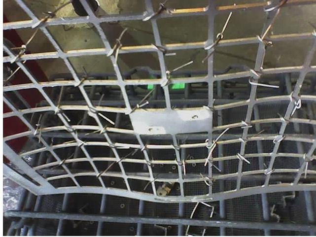
Figure 5 - Fixture After Creep
