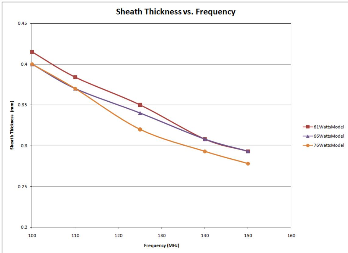
**Figure 3.2 Model predictions for Sheath thickness vs. frequency**
