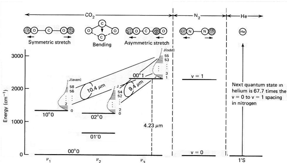
**Figure 1.1 Laser process in a CO<sub>2</sub>:N<sub>2</sub>:He gas laser**
