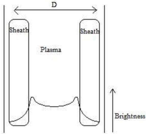
**Figure 1.3 Ion sheath and visible emission**
