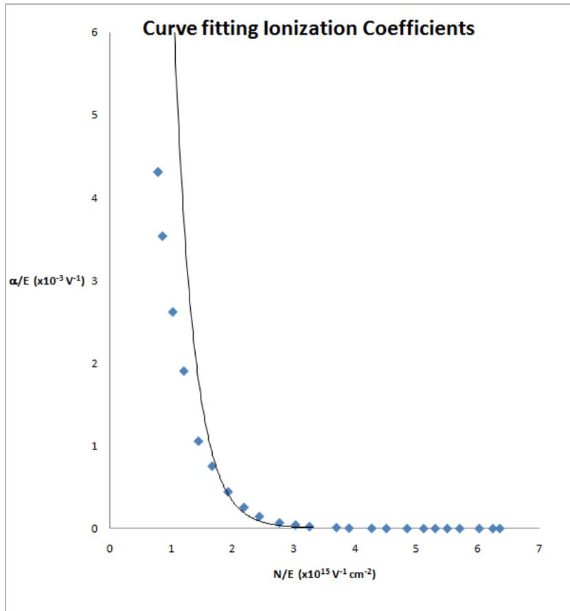
**Figure 2.1 Curve fitting used to find Townsend Coefficient**
