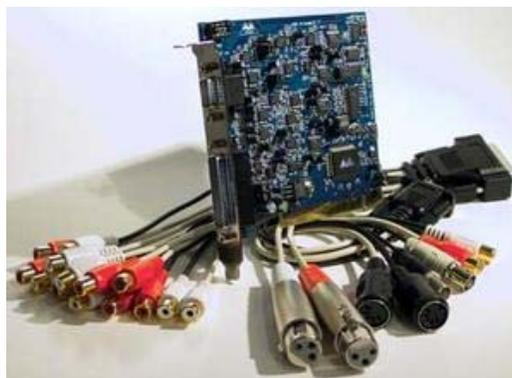
**Figure 4 - PCI 10 Input/Output Sound Card (American)**
