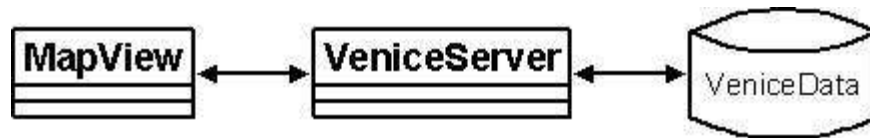
Figure 3: The initial design of the Venice mapping Web application. MapView represents the Web-based mapping application front end, and VeniceServer represents the data model that will be used by MapView. The arrows signify the flow of information, not dependencies or relationships.
