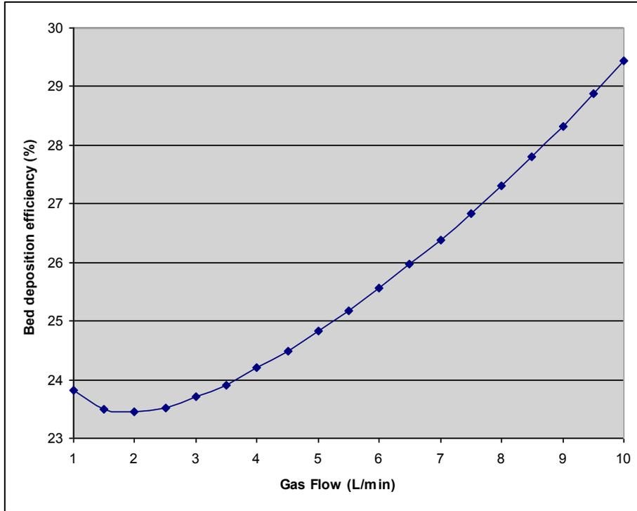
Figure 2.5.7. Effect of gas flow rate on bed deposition efficiency for  $\alpha = 0.19$ .
