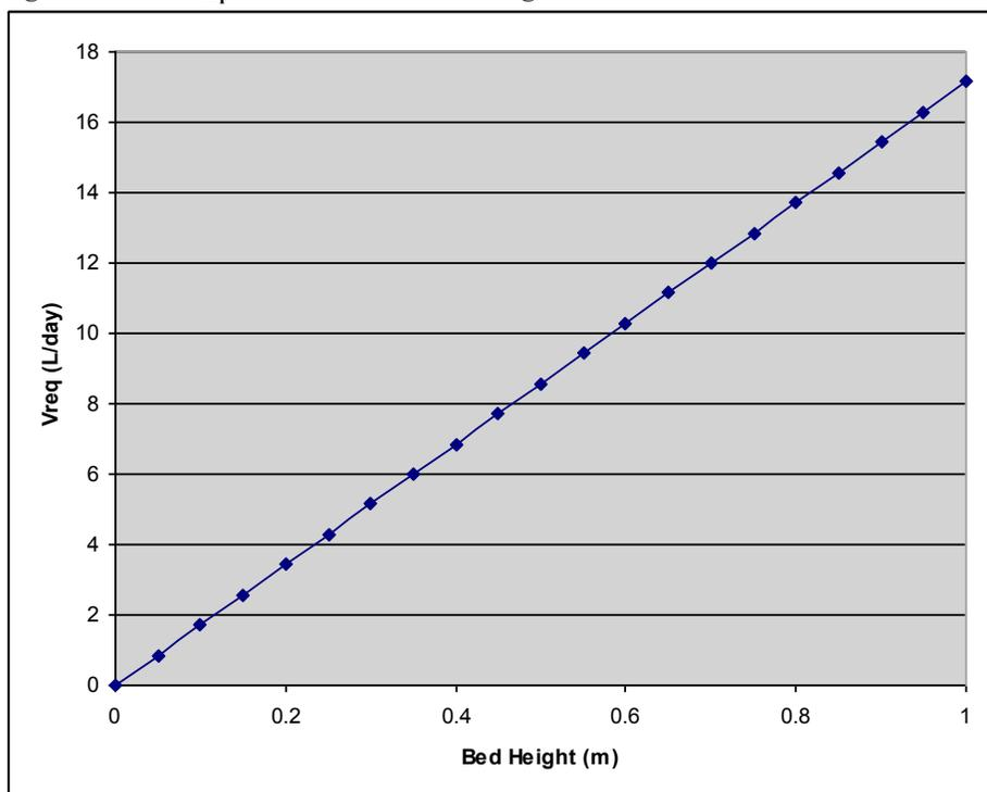
Figure 2.5.3d.  $V_{req}$  as a function of bed height for  $\alpha=0.71$ .
