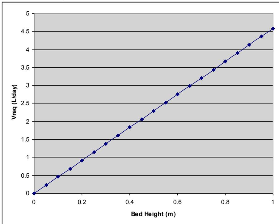
Figure 2.5.3b.  $V_{req}$  as a function of bed height for  $\alpha=0.19$ .
