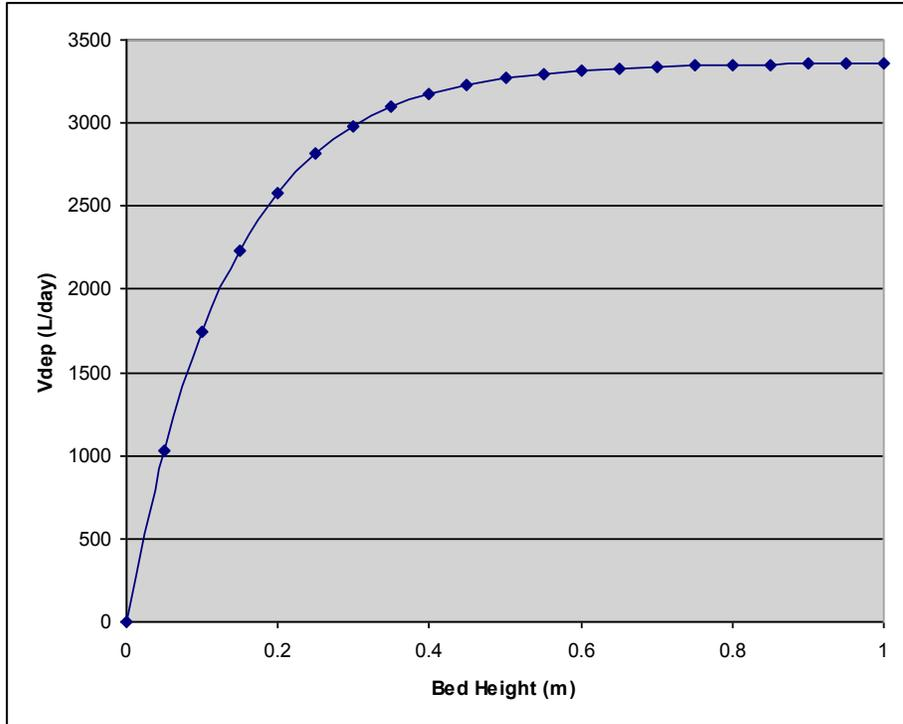
Figure 2.5.3a.  $V_{dep}$  as a function of bed height for  $\alpha=0.19$ .
