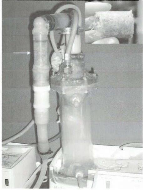
**Figure 2.4.3. Nutrient mist bioreactor used by Towler, et al. (2006), and a harvested root mass they were able to achieve ( $\alpha=0.71$ ). Arrow indicates growth culture chamber.**
