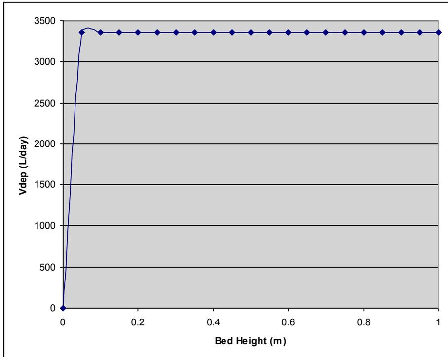
Figure 2.5.3c.  $V_{dep}$  as a function of bed height for  $\alpha=0.71$ .
