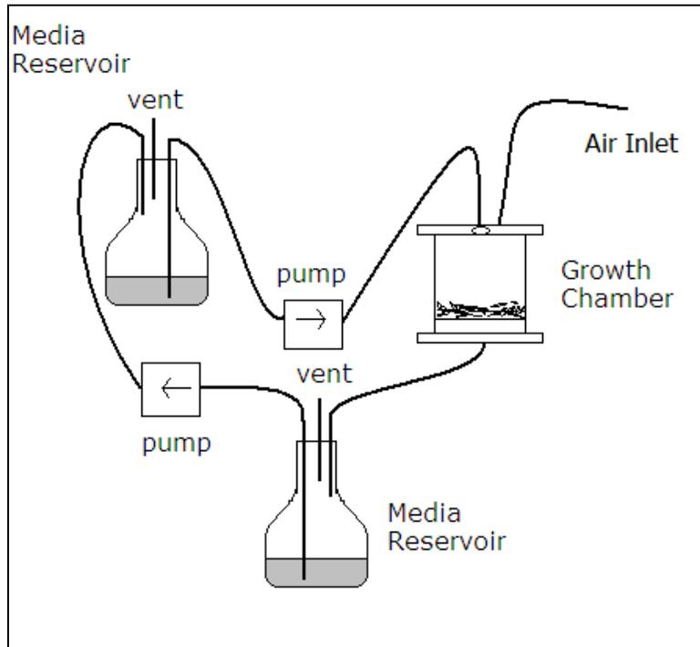
Figure 2.5.1. Schematic of my reactor.
