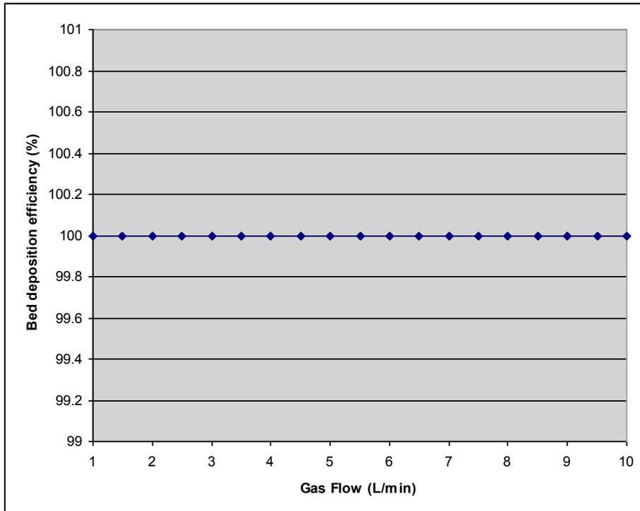
Figure 2.5.8. Effect of gas flow rate on bed deposition efficiency for  $\alpha = 0.71$ .
