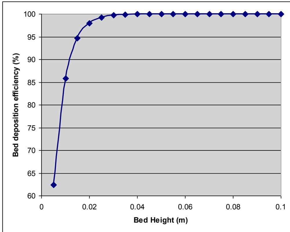
Figure 2.4.1. Effects of bed height on mist deposition at  $\alpha=0.5$ .
