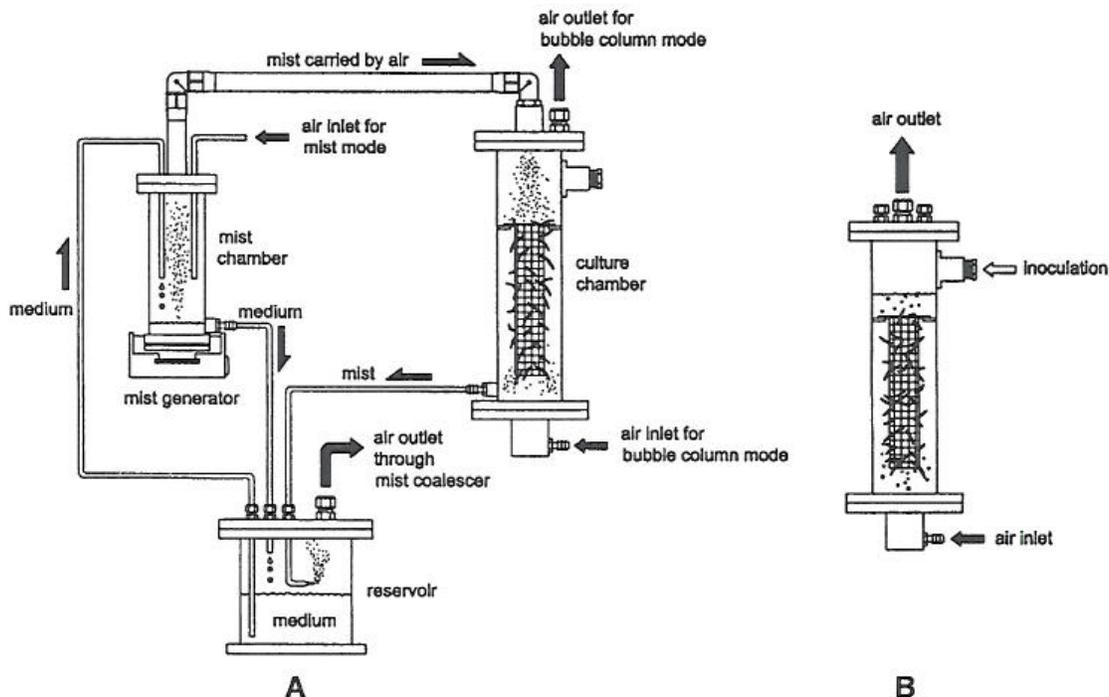
Figure 2.4.2. Mist reactor (A) and bubble column (B) used by Kim, et al. (2001)
