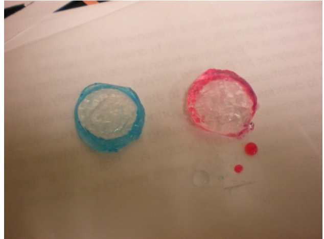
Figure 17 - PAA/PVA samples after coatings applied
