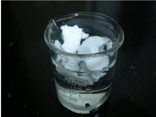
Figure 16 - Dissolving Styrofoam(Polystyrene) in acetone
