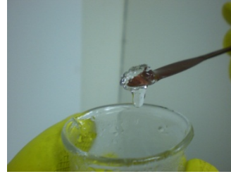
Figure 2 – PAA Hydrogel taking shape after undergoing Thermal Crosslinking
