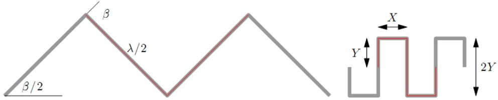
Figure 2: Sawtooth and square. Here the slope angle of the sawtooth is  $\alpha = \pi/4$ , and  $X = Y/2 = \lambda/6$ . The light gray curve in the background shows the continuation of the waveform.
