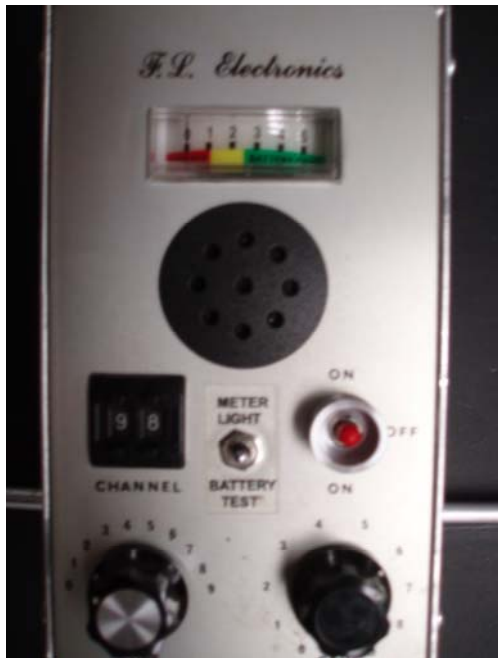
Figure 17: Close Up of Radio Control Box
