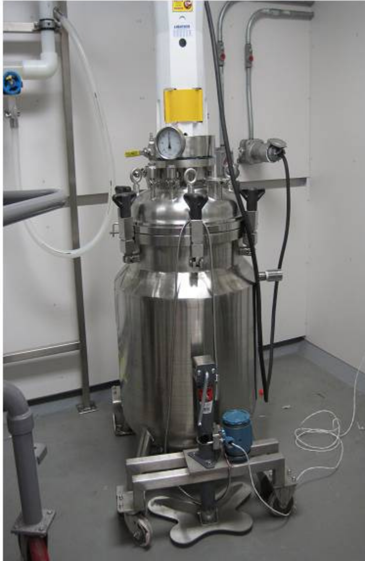
Figure 4: The 30 gallon stainless steel vessel used for the polymerization phase
