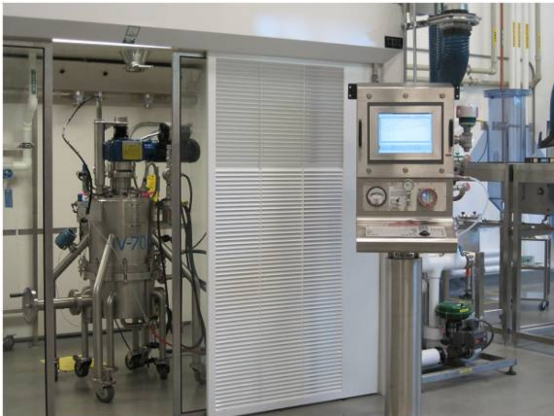
Figure 1: The DeltaV interface in the pilot plant and the 0.1 m Nutsche reactor in the walk-in hood
