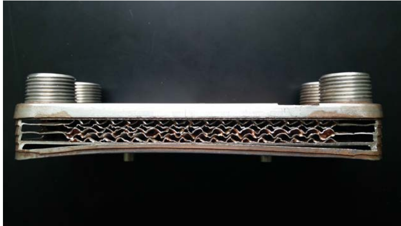
Figure. 5 Side View of the Installed Plate Heat Exchanger
