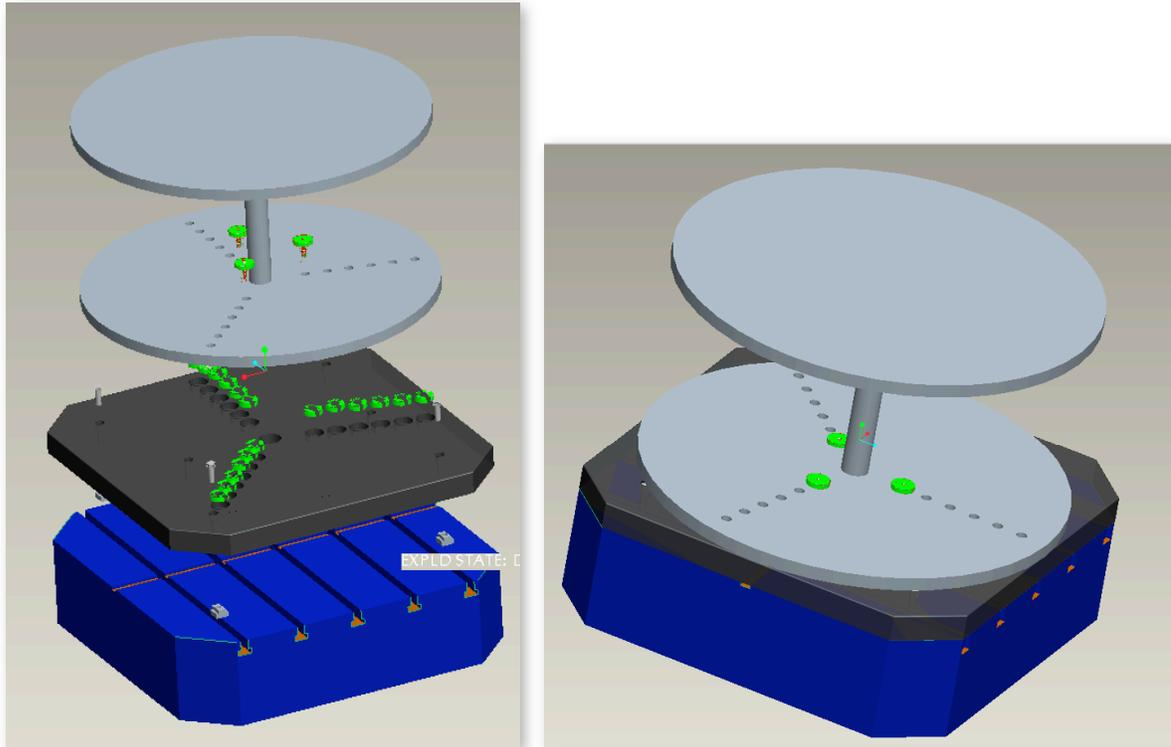
Figure 4.5: Fixturing System Mock-Up Exploded and Assembled View
