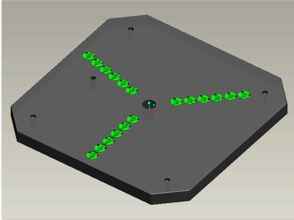
*Figure 4.2: Proposed Sub-plate Design and Hole Pattern*
