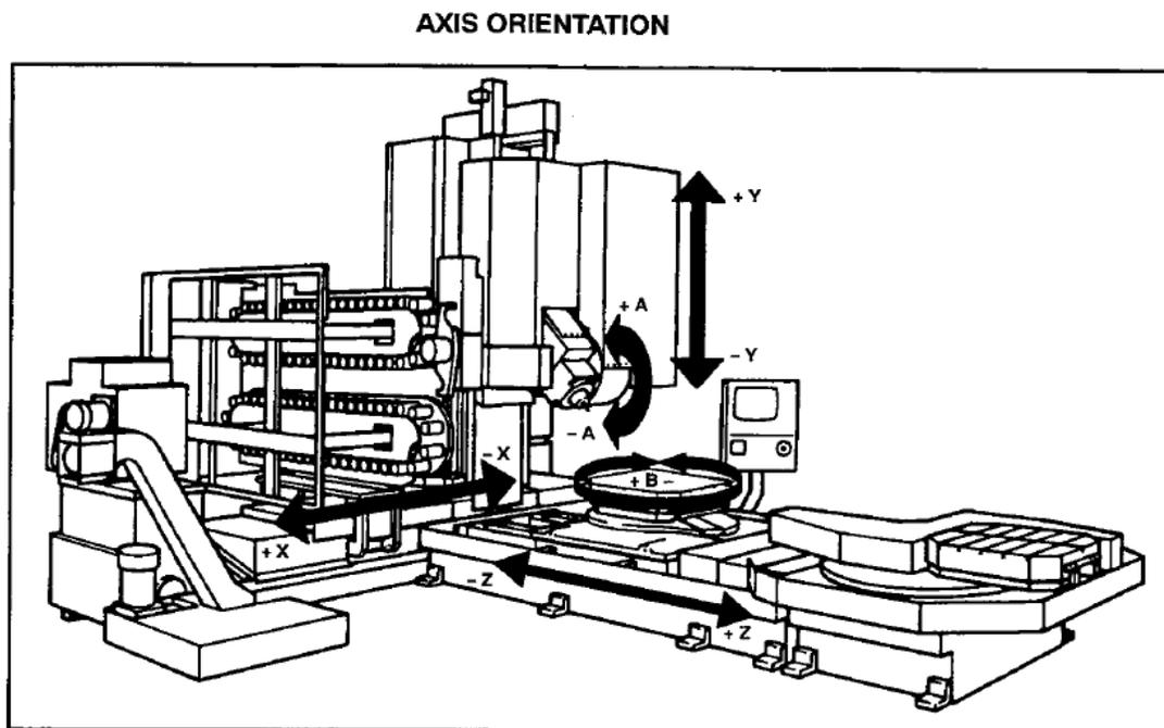
Figure 2.1: The Axis Orientations on the Cincinnati T35
