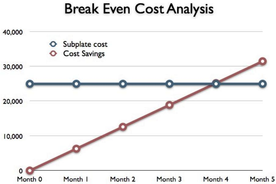
Figure 4.6: Break Even Cost Analysis of Sub-plate Design
