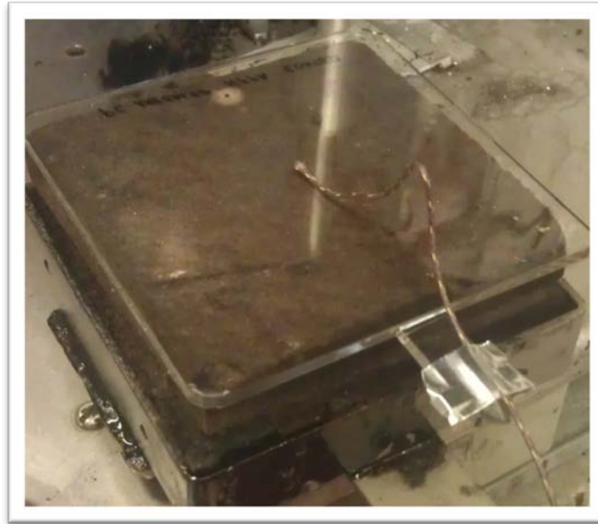
Figure 17: Thermocouple Attached to Center of Plaque
