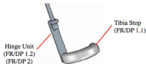
Figure 6: Image of FRs/DPs 1.1 and 1.2 in our design.
