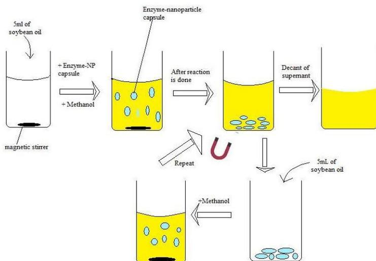
*Figure 7: Process for Biodiesel Production Using ENP*
