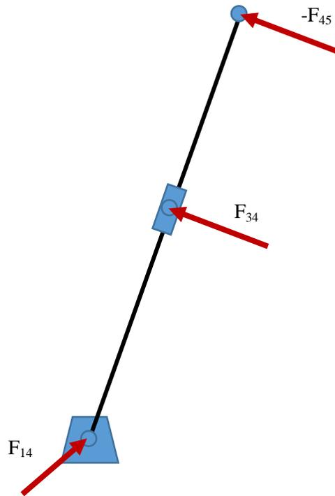
Figure 5: Free body diagram of link 4.
