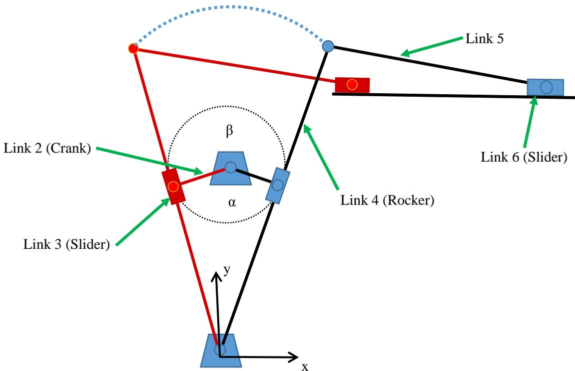
Figure 2: Basic design of a Crank-Shaper 6 Bar Mechanism
