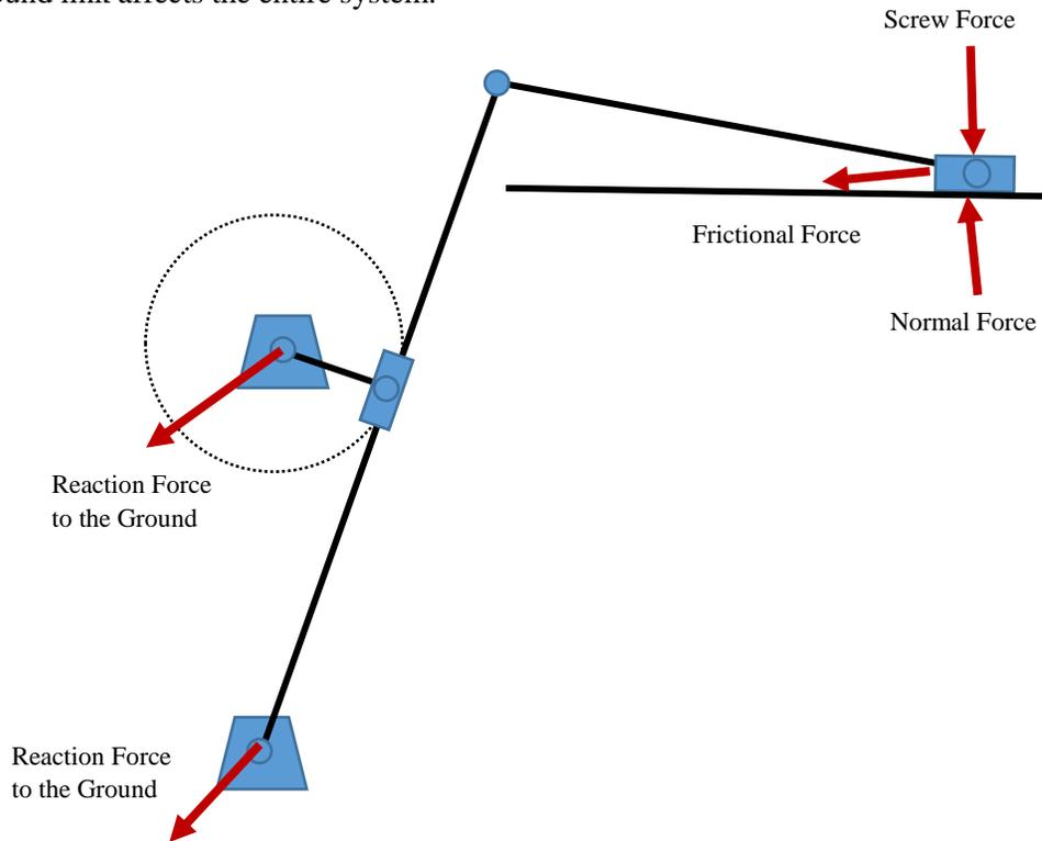
Figure 6: Overall Free Body Diagram of the Mechanism
