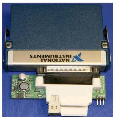
**Figure-1: Analog Input Module and Bumper**
