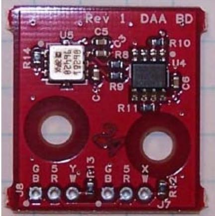
**Figure-3: Dual Axis Accelerometer**
