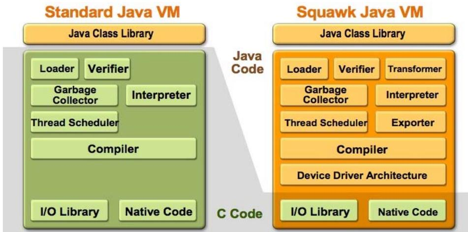
Figure-6: the Standard Java Virtual Machine vs. the Squawk Virtual Machine
